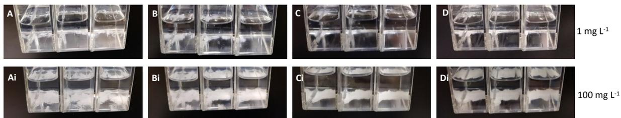
**Figure SI.4.** Photographic observation of sedimentation of nTiO<sub>2</sub> triplicate samples during DLS analysis; A/Ai – 24 h, B/Bi – 168 h, C/Ci – 240 h, D/Di – 336 h.
