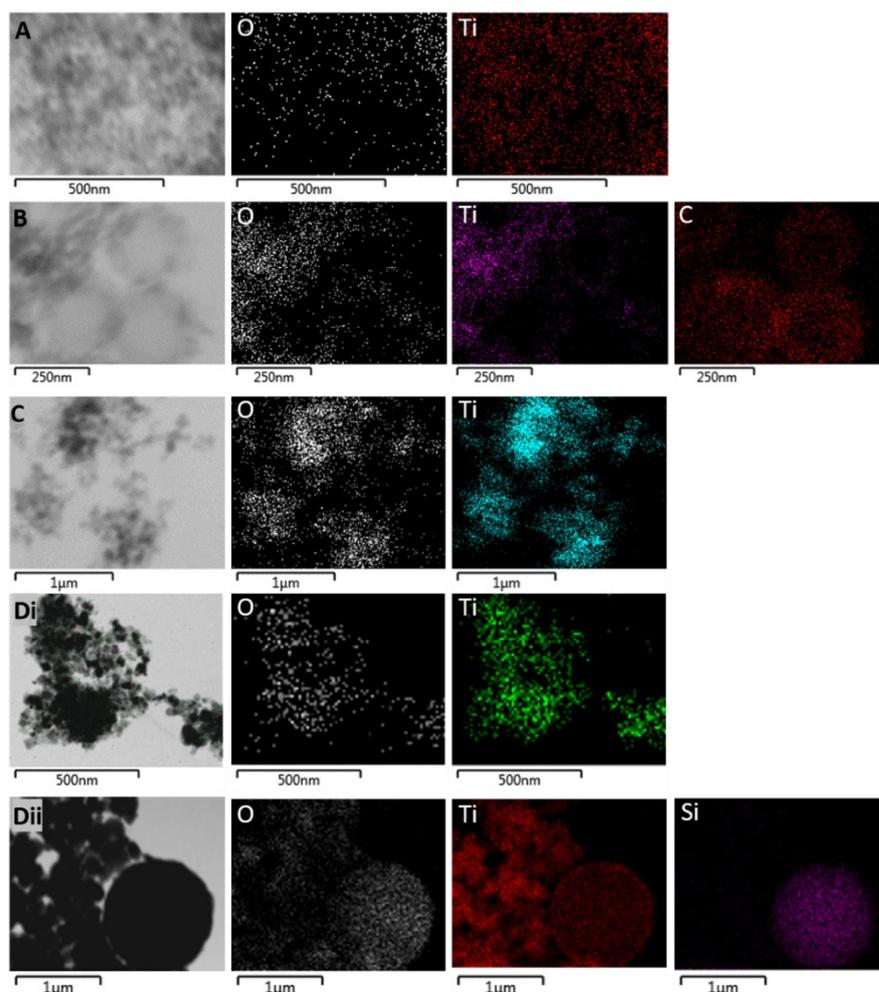
**Figure SI.1.** A – research-grade nTiO<sub>2</sub> nanopowder purchased from Sigma Aldrich; B – nTiO<sub>2</sub> extracted from Skinceuticals™ sunscreen (S1); C – nTiO<sub>2</sub> extracted from Boots Soltan™ sunscreen (S2); Di and Dii – nTiO<sub>2</sub> extracted from The Body Shop™ liquid foundation (P1). Left panel shows scanning transmission electron microscope image of samples; other panels show false coloured EDS image of element as labelled.
