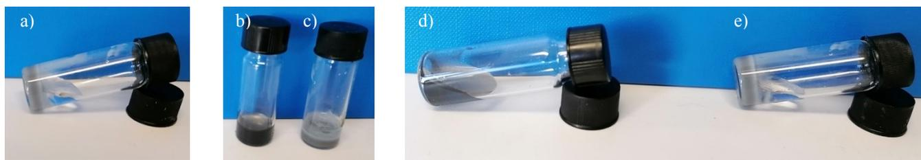
**Figure S3.** Pictures of **a)** water in contact with hybrid gels after adsorption, **b-d)** dispersion of graphite in water, **c-e)** water in contact with **graphite/PF<sub>6</sub>** gel after 5h.
