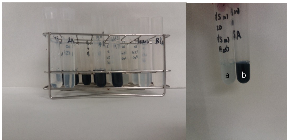
Figure A.2: Lowry method modified by Peterson applied to: a) samples without allylthiourea (ATU); b) samples with ATU.
