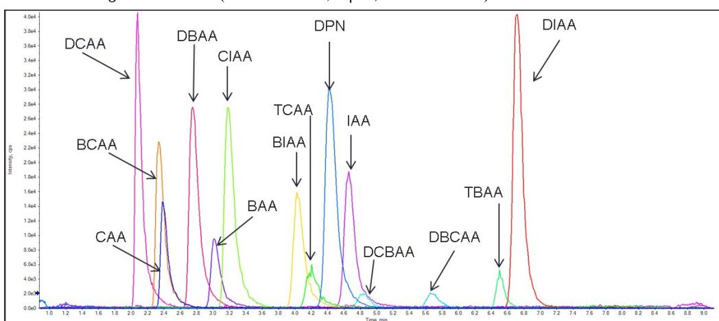
**Figure S2.** Chromatographic resolution of HAA peaks after LVI (200  $\mu$ l)-LC-ESI(-)-HRMS of an HPLC-grade water containing 30  $\mu$ g/L of the HAAs mix in the two LC columns tested. A mobile phase consisting of ACN: H<sub>2</sub>O, both with 0.1% formic acid, was used in both injections.
