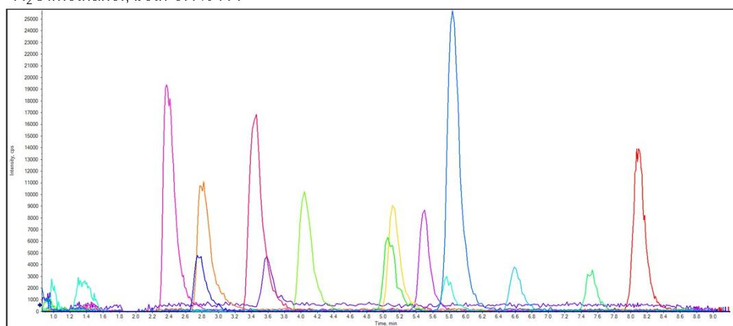
**Figure S3.** Chromatographic separation of HAAs (25 µg/L) in the Lunar Omega Polar C18 column using different mobile phase compositions: methanol or acetonitrile as organic constituent.
