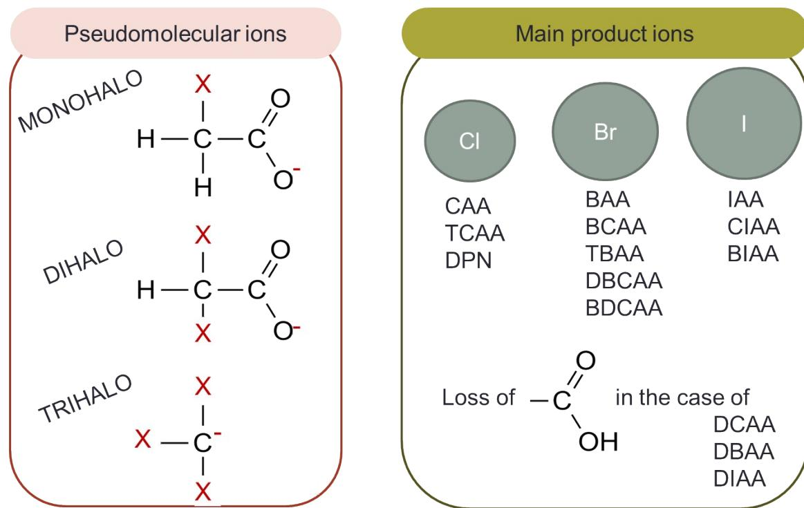
**Figure S1.** Formation of pseudomolecular ions and main product ions of HAAs under electrospray negative ionization.
