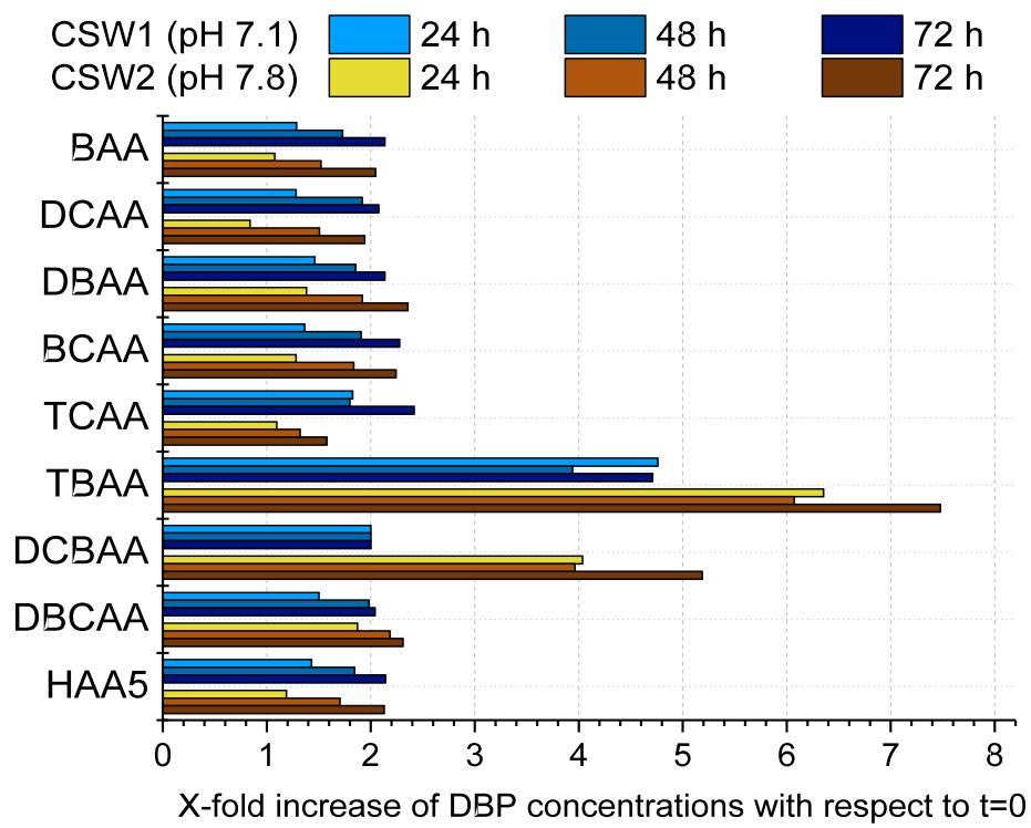
**Figure S5.** X-fold increase of DBP concentrations at different reaction times with respect to t=0, calculated as  $C_t/C_0$ , where  $C_t$  is the concentration at time = 24 h, 48 h or 72 h and  $C_0$  is the concentration at time =0.
