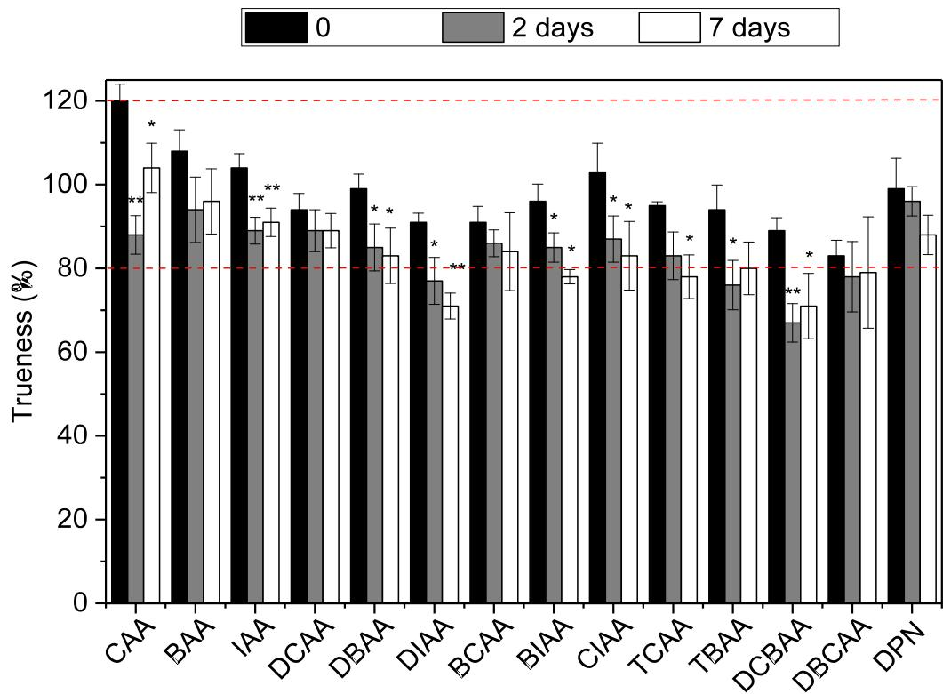
**Figure S4.** Average trueness of HAA measurements in HPLC-grade water samples (n=3) fortified at a concentration of 5 µg/L and after two and seven days stored at -20°C in the dark. Error bars indicate RSD values of n=3 independently prepared and analyzed samples.
