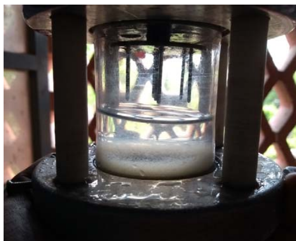
Fig. S3. Reactor with flocs settled at bottom
