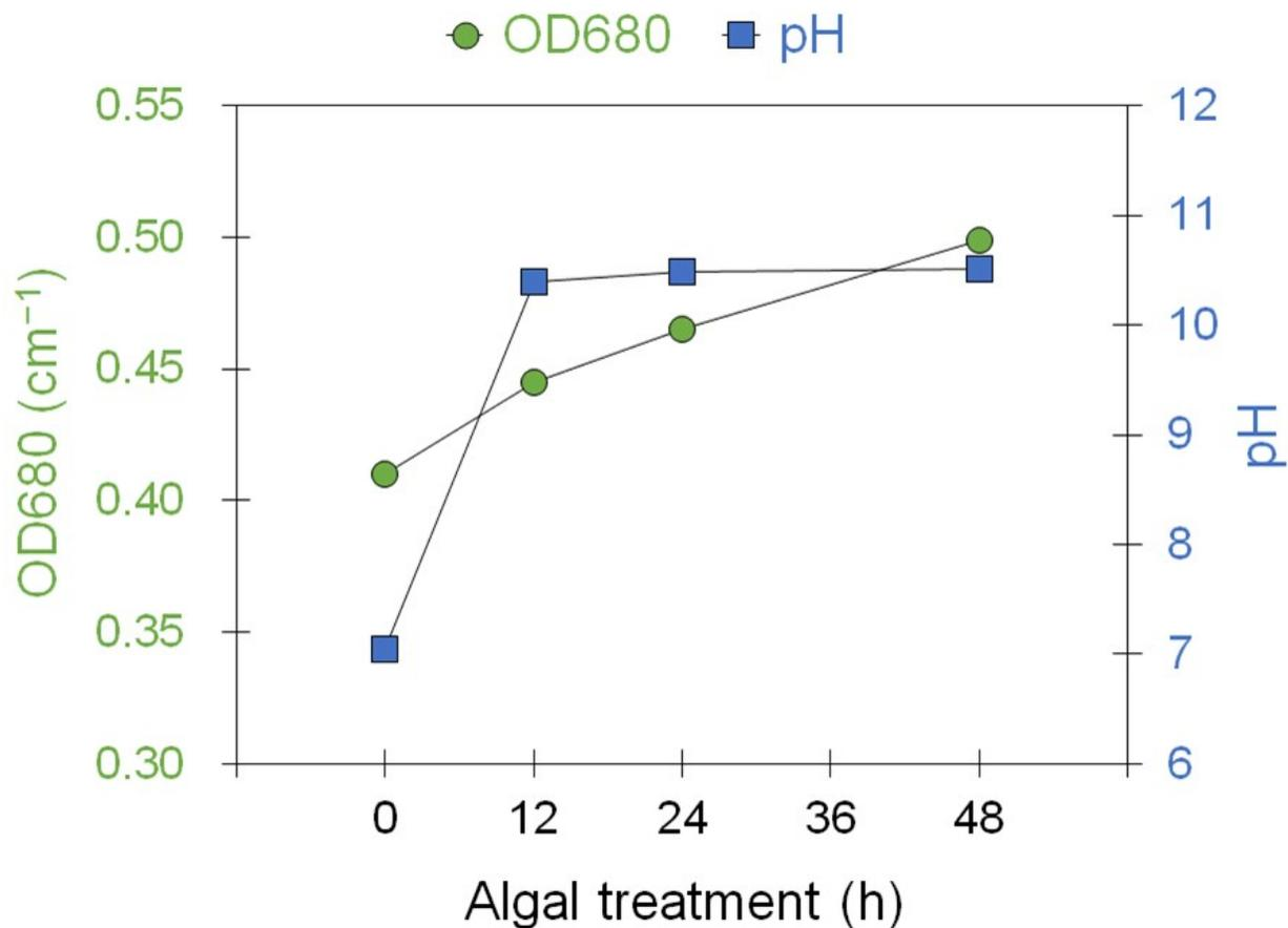
Fig. S2. The growth of algal biomass and the associated pH increase in livestock wastewater effluent. A microalga *Scenedesmus quadricauda* was incubated in the light for 48 h without supplemented CO<sub>2</sub>. The cell growth was measured by monitoring the optical density at 680 nm (OD680).
