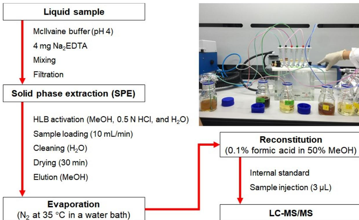
Fig. S1. Sample preparation (extraction and clean-up) procedure for LC-MS/MS analysis of selected antibiotics.
