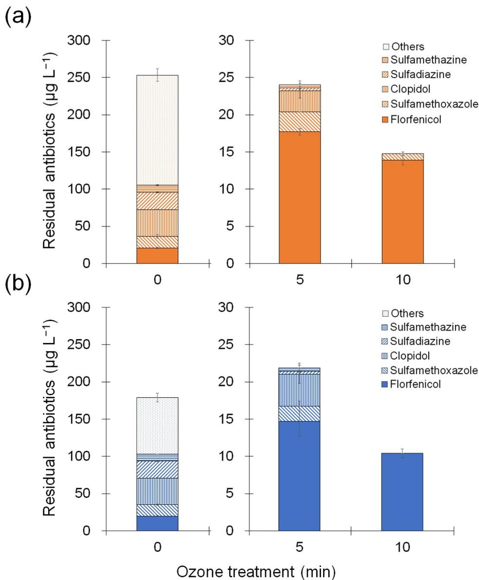
Fig. S6. The effects of ozonation on the removal of antibiotics from raw neutral (a) and algal-treated alkaline (b) livestock wastewater. The ozonation of raw and algal-treated livestock wastewater was carried out for up to 10 min (equivalent to  $\sim 1.8 \text{ mg-O}_3/\text{mg-C}$ ). Fig. 8a in the main text was reconstructed here in terms of clopidol, florfenicol, sulfadiazine, sulfamethazine, and sulfamethoxazole. The other antibiotics were not detected in the ozonated wastewater.
