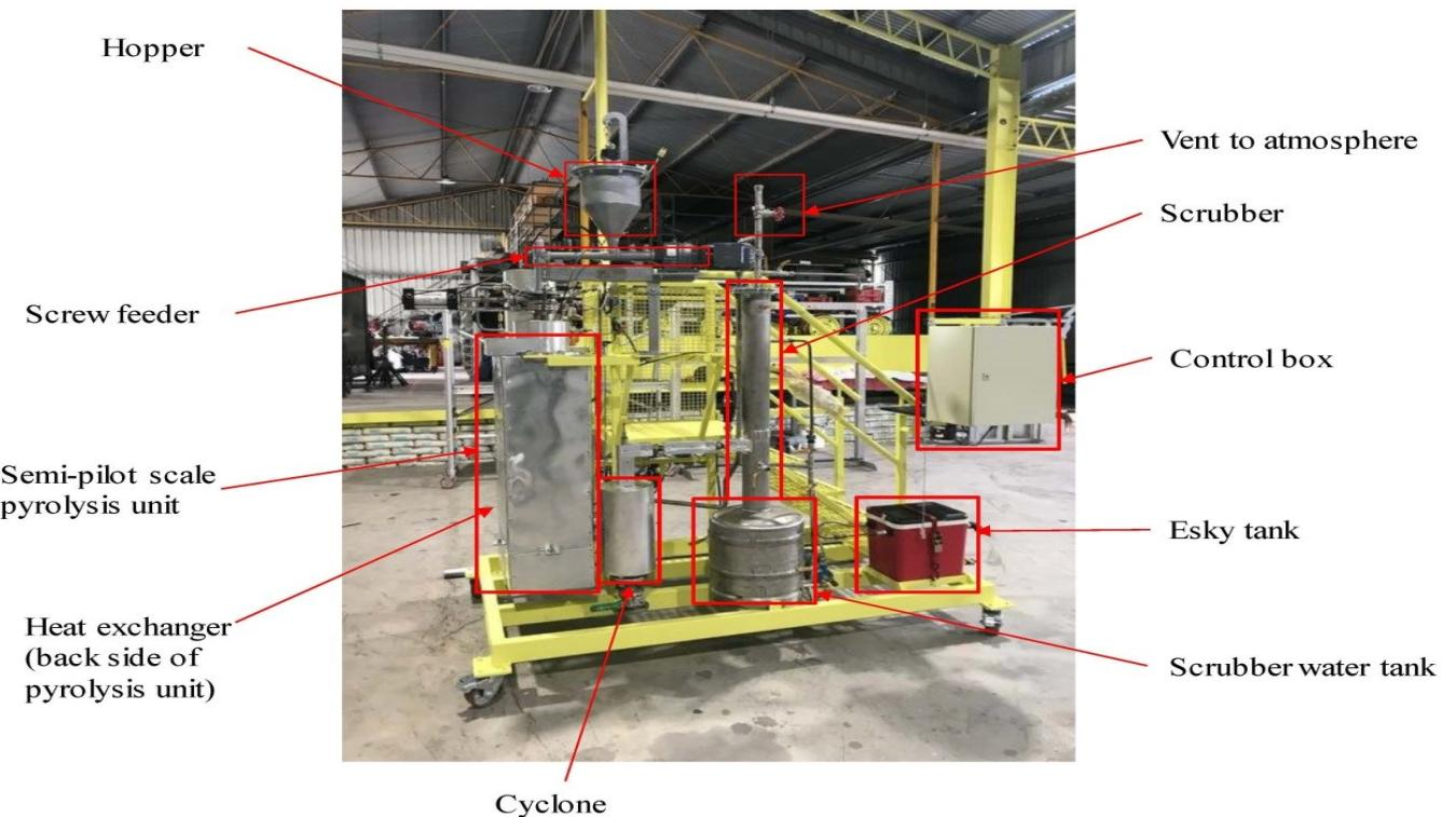
**Figure S2:** Semi-pilot plant for biosolids' pyrolysis trials.
