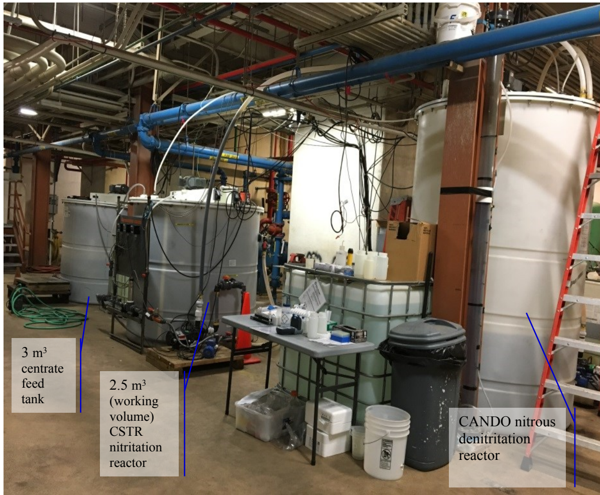
Figure S2. Pilot-scale nitritation reactor at the Delta Diablo wastewater treatment plant.
