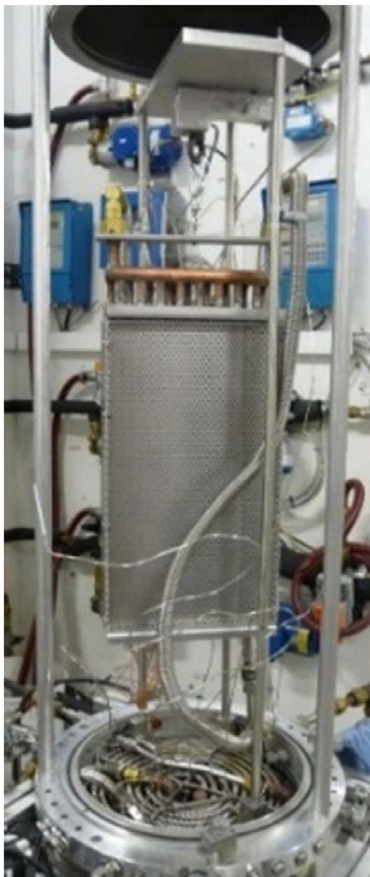
Figure S1: Open single chamber with suspended heat exchanger (adsorber-desorber) and evaporator-condenser (e/c) underneath.
