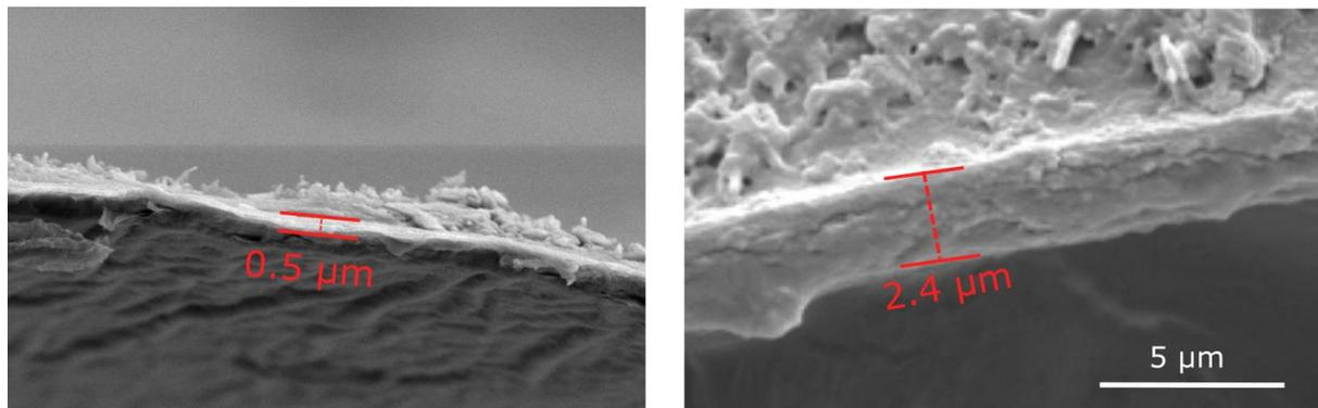
**Fig. 58** SEM images of a cross section of the adaxial side of a *Tradescantia* leaf. In each image the thickness of the cell wall is indicated, showing large differences in local thickness.
