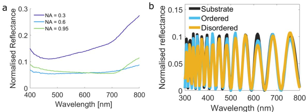
**Fig. S6** a) Optical microscope spectra for several numerical apertures, showing that for a larger angular detection range the long wavelength increase is obscured. b) 2D FDTD calculation of the total reflection of the bare substrate, the substrate plus a collection of ordered platelets and the substrate plus a collection of disordered platelets.
