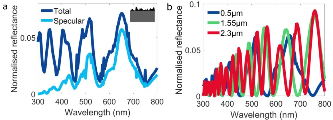
**Fig. 57** Two dimensional FDTD calculations of a) Total and specular reflection from a rough surface, and d) specular reflection of disordered platelets with varying substrate thickness.
