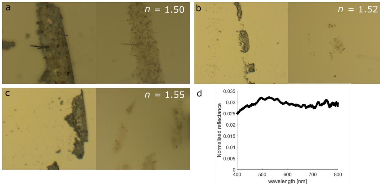
**Fig. S5** a), b) and c) Optical microscope images of wax platelets that have been removed from a leaf before (left) and after (right) adding refractive index matching oils. The wax platelets almost fully disappear upon addition of oil of  $n = 1.52$ . b) Specular reflectance as measured using an integrating sphere. The average value over 400 to 800 nm range is used in Fresnel equation to calculate the refractive index of the substrate.
