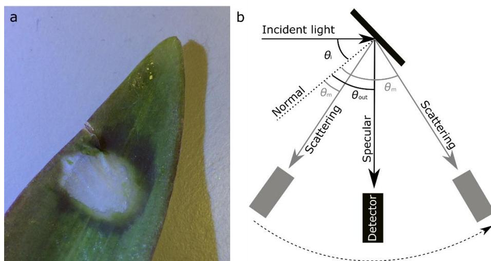
**Fig. S1** a) *Tradescantia* leaf with locally removed subepidermal layers. b) Sketch of a goniometer setup with  $\theta_m$  the angle of incidence for light illuminating the sample,  $\theta_m$  the scattering angle and  $\theta_{out}$  the specular reflection angle.
