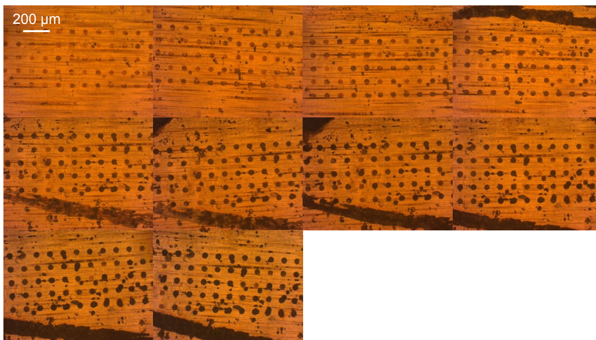
Figure S91: Platinum time series for sample prepared with 2 layers of CMC and 2% PMMA spin-coated for 1 minute at 1000 rpm. Images were taken after electroplating for 30 s, 60 s, 90 s, 120 s, 150 s, 180 s, 210 s, 240 s, 300 s, and 360 s.
