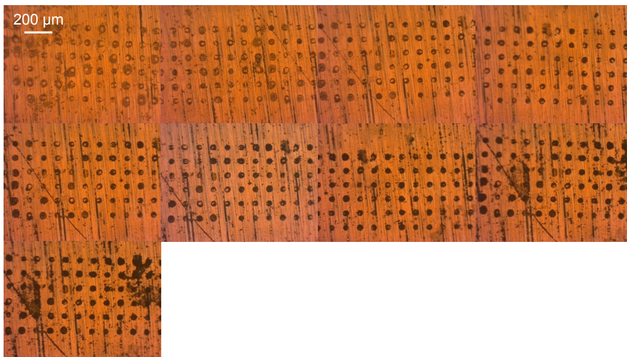
Figure S103: Platinum time series for sample prepared with 4 layers of CMC and 2% PMMA spin-coated for 1 minute at 4000 rpm. Images were taken after electroplating for 30 s, 60 s, 90 s, 120 s, 150 s, 180 s, 240 s, 300 s, and 360 s.
