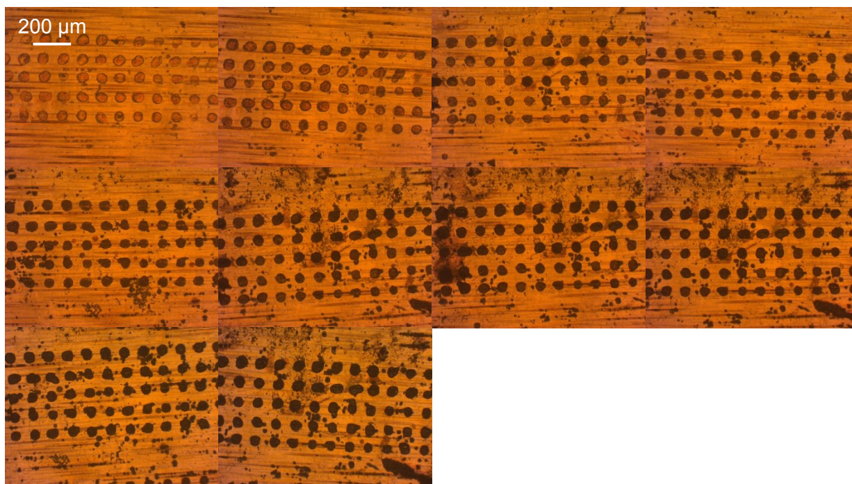
Figure S94: Platinum time series for sample prepared with 5 layers of CMC and 2% PMMA spin-coated for 1 minute at 1000 rpm. Images were taken after electroplating for 30 s, 60 s, 90 s, 120 s, 150 s, 180 s, 210 s, 240 s, 300 s, and 360 s.
