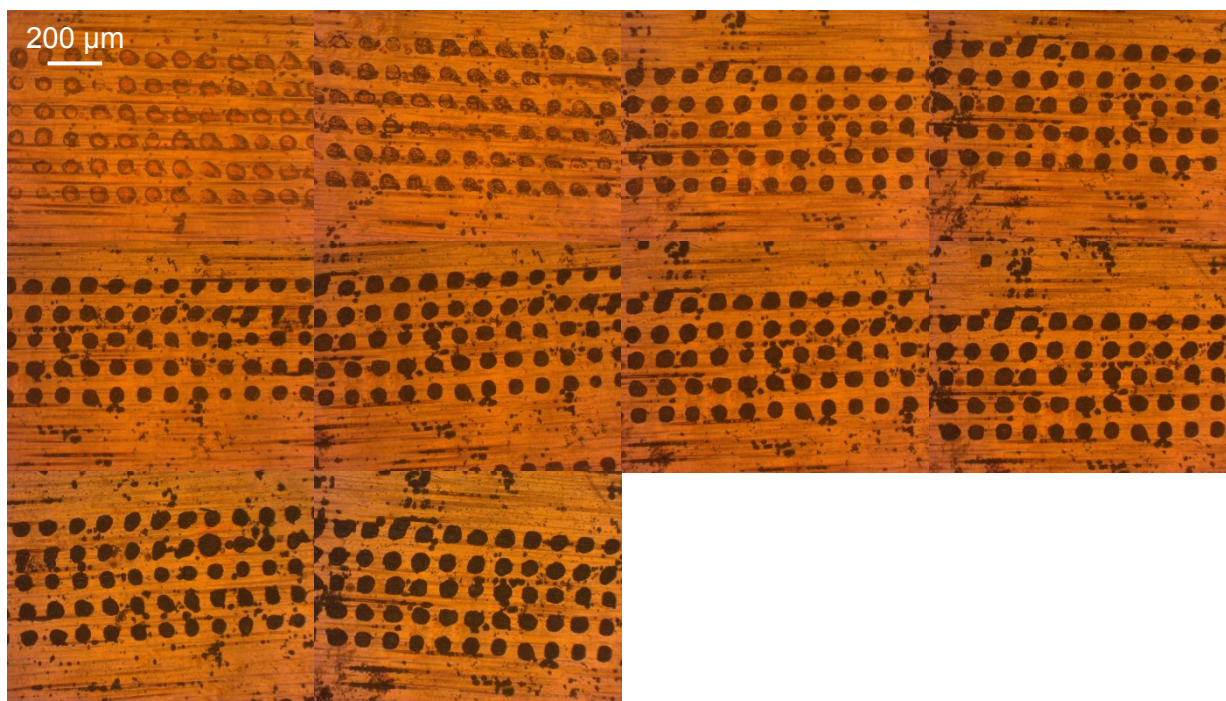
Figure S95: Platinum time series for sample prepared with 6 layers of CMC and 2% PMMA spin-coated for 1 minute at 1000 rpm. Images were taken after electroplating for 30 s, 60 s, 90 s, 120 s, 150 s, 180 s, 210 s, 240 s, 300 s, and 360 s.
