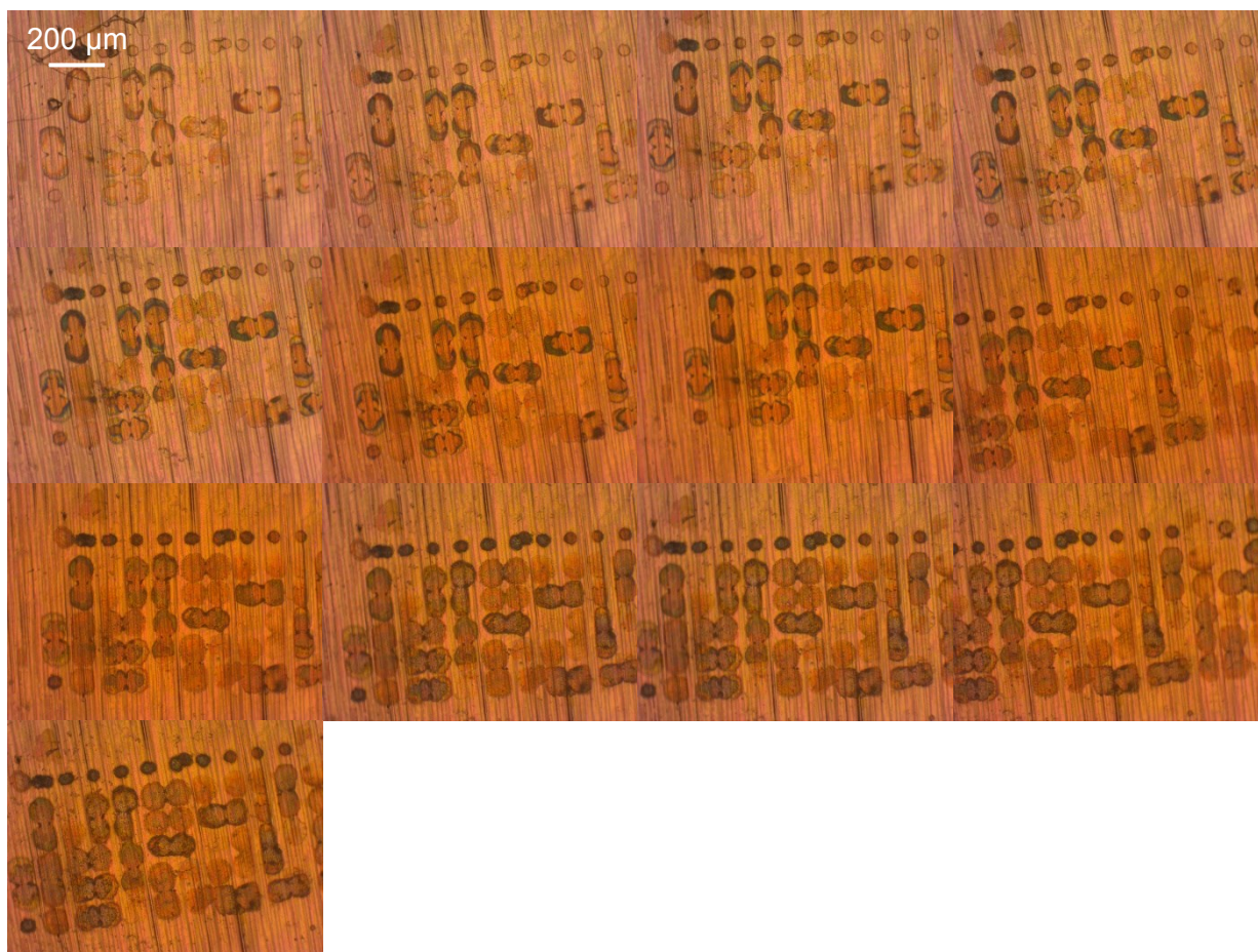
Figure S113: Platinum time series for sample prepared with 4 layers of CMC and 7% PMMA spin-coated for 1 minute at 4000 rpm. Images were taken after electroplating for 15 s, 30 s, 45 s, 60 s, 90 s, 120 s, 150 s, 180 s, 210 s, 240 s, 270 s, 300 s, and 360 s.
