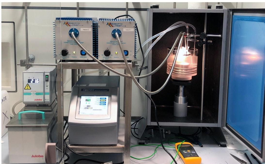
**Figure s1.** The experimental setup of the SonoPhotoReactor.
