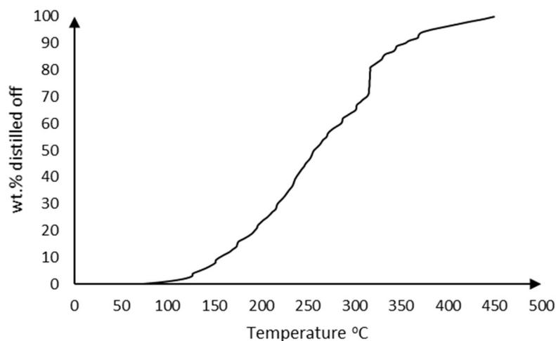
**Figure S3.** Simulated distillation of the bio-oil
