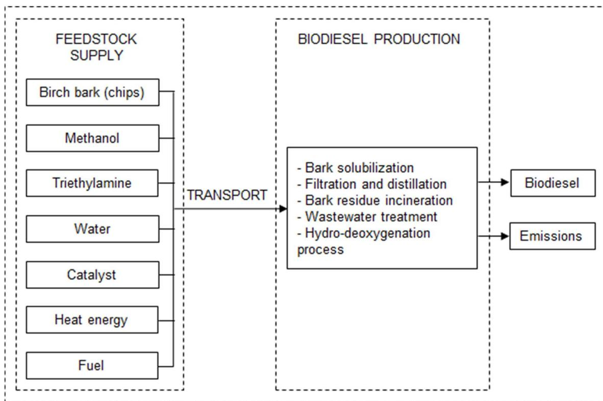
**Figure S5.** Cradle to gate system boundary of the biodiesel production
