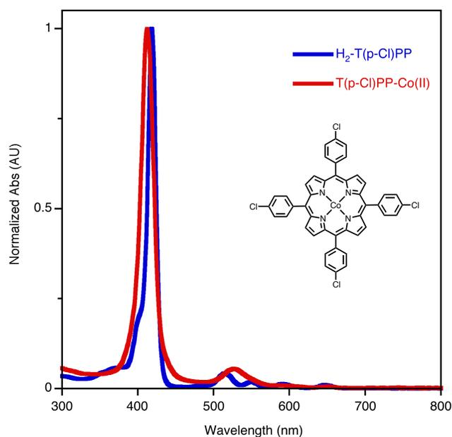
**Figure S18.** UV-vis spectrum (CH<sub>2</sub>Cl<sub>2</sub>) of [T(p-ClP)P]Co in comparison to that of the corresponding free base T(p-ClP)P.
