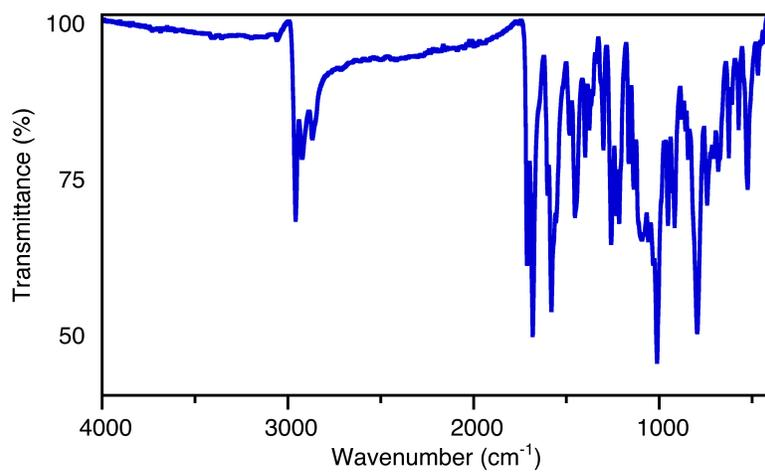
**Figure S8:** FT-IR spectrum (neat, diamond ATR) of [2,7-dioxo-OEP]Co.
