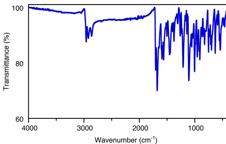
**Figure S11:** FT-IR spectrum (neat, diamond ATR) of **[2,12-dioxo-OEP]Co**
