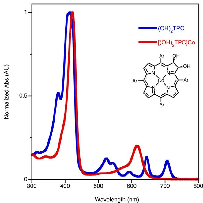
**Figure S30.** UV-vis spectrum ( $\text{CH}_2\text{Cl}_2$ ) of  $[(\text{OH})_2\text{TPC}]\text{Co}$  in comparison to that of the corresponding free base  $(\text{OH})_2\text{TPC}$ .  $[(\text{OH})_2\text{TPC}]\text{Co}$  is literature-known.<sup>5</sup>
