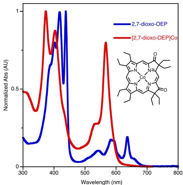
**Figure S6.** UV-vis spectrum ( $\text{CH}_2\text{Cl}_2$ ) of **[2,7-dioxo-OEP]Co** in comparison to that of the corresponding free base **2,7-dioxo-OEP**. **[2,7-dioxo-OEP]Co** is reported here firstly.
