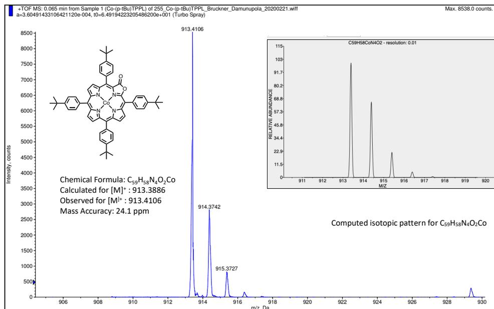
Figure S23. ESI+ HR-MS (100%  $CH_3CN$ , TOF) of  $[T(p\text{-}tBuP)L]Co$ .
