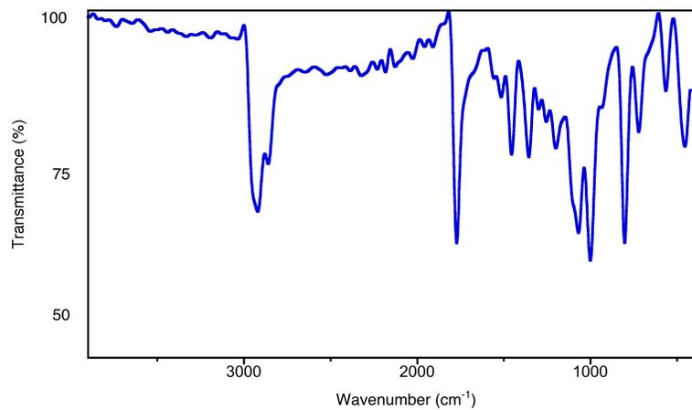
Figure S24. FT-IR spectrum (neat, diamond ATR) of  $[T^FPL]Co$ .
