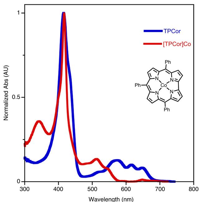
**Figure S33.** UV-vis spectrum ( $\text{CH}_2\text{Cl}_2$ ) of [TPCor]Co in comparison to that of the corresponding free base TPCor. [TPCor]Co is literature-known.<sup>7</sup>
