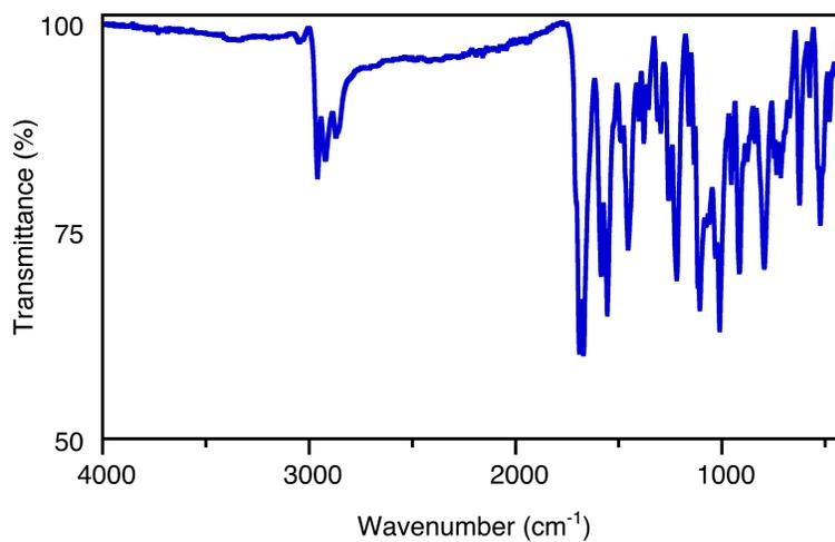
**Figure S14:** FT-IR spectrum (neat, diamond ATR) of **[2,7,18-trioxo-OEP]Co**
