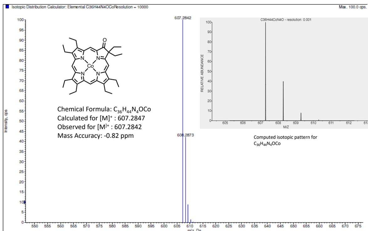
**Figure S4.** ESI+ HR-MS (100% CH<sub>3</sub>CN, TOF) of [2-oxo-OEP]Co.
