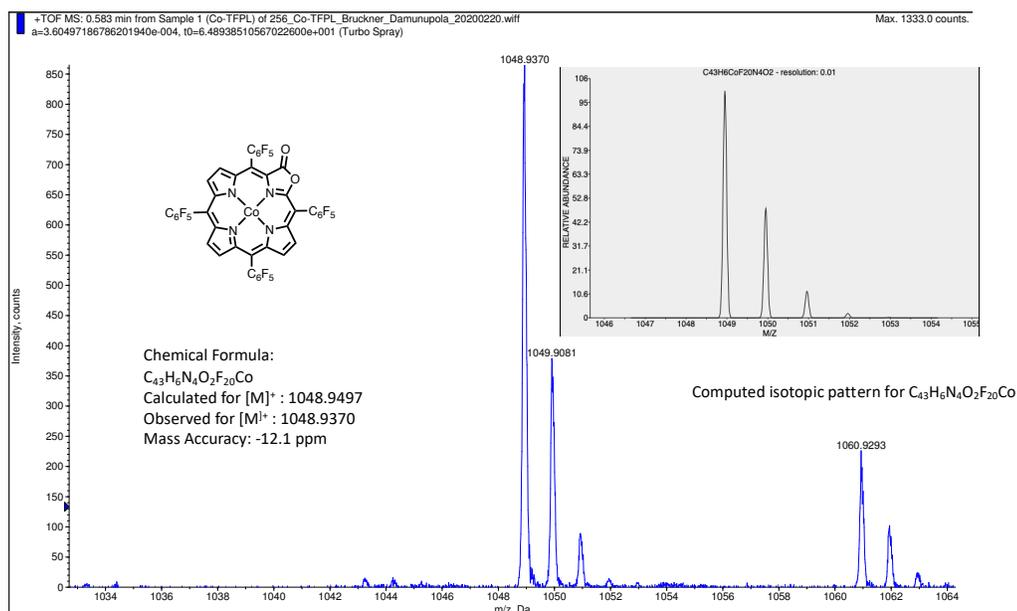
**Figure S20.** ESI+ HR-MS (100%  $CH_3CN$ , TOF) of  $[T^FPL]Co$ .
