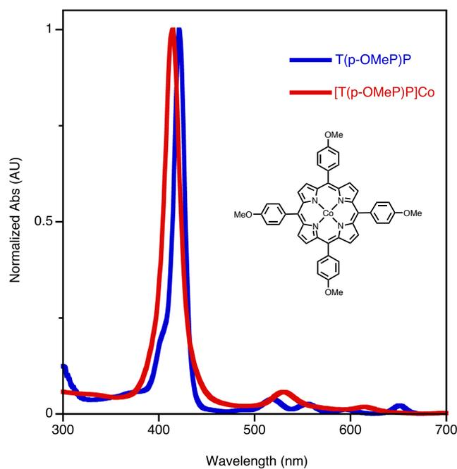
**Figure S17.** UV-vis spectrum (CH<sub>2</sub>Cl<sub>2</sub>) of [T(p-OMeP)P]Co in comparison to that of the corresponding free base T(p-OMeP)P. [T(p-OMeP)P]Co is literature-known.<sup>3</sup>
