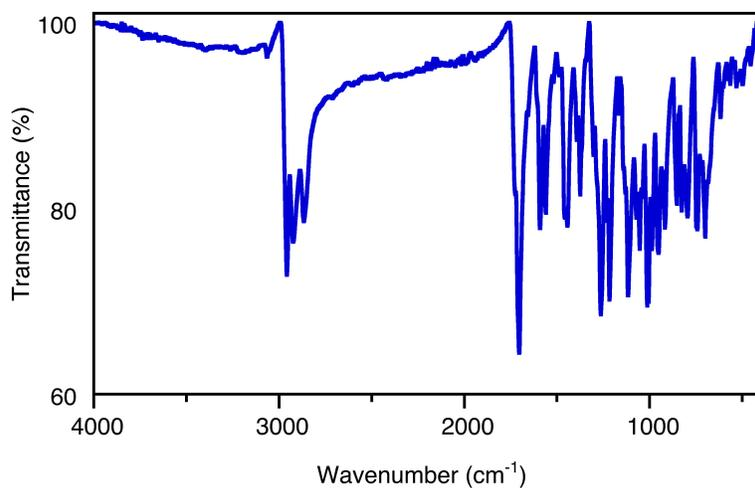
**Figure S5:** FT-IR spectrum (neat, diamond ATR) of **[2-oxo-OEP]Co**.
