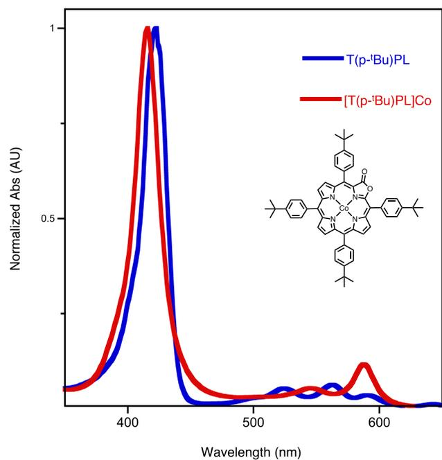
**Figure S22.** UV-vis spectrum ( $CH_2Cl_2$ ) of  $[T(p\text{-}^tBuP)L]Co$  in comparison to that of the corresponding free base  $T(p\text{-}^tBuP)L$ .  $[T(p\text{-}^tBuP)L]Co$  reported here firstly.
