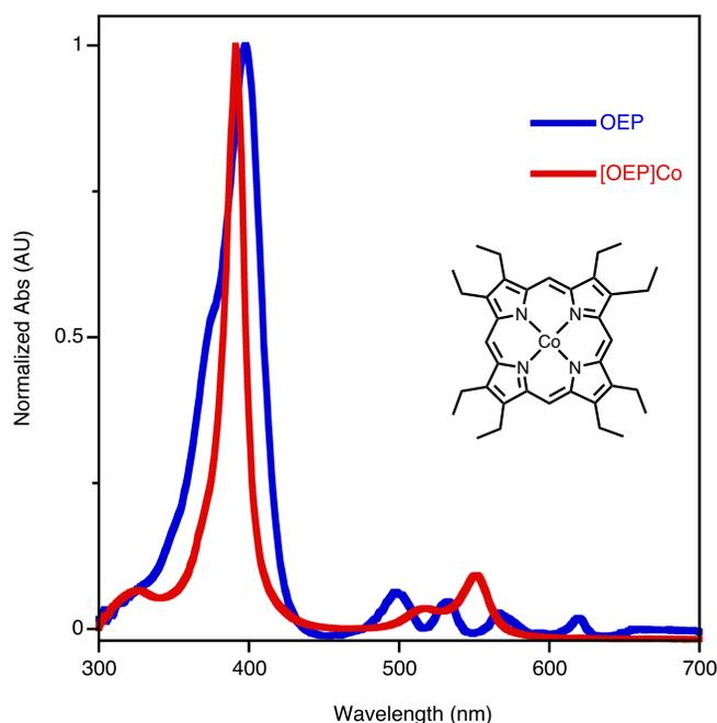
**Figure S1.** UV-vis spectrum (CH<sub>2</sub>Cl<sub>2</sub>) of **[OEP]Co** in comparison to that of the corresponding free base **OEP**. **[OEP]Co** is literature-known.<sup>1</sup>
