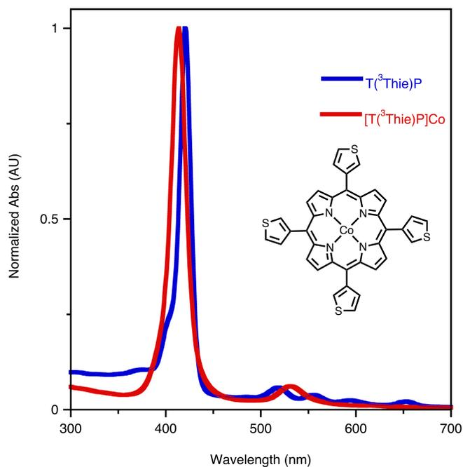
**Figure S25.** UV-vis spectrum (CH<sub>2</sub>Cl<sub>2</sub>) of [T<sup>3</sup>Thie)P]Co in comparison to that of the corresponding free base T(3Thie)P. [T<sup>3</sup>Thie)P]Co is literature-known.<sup>4</sup>
