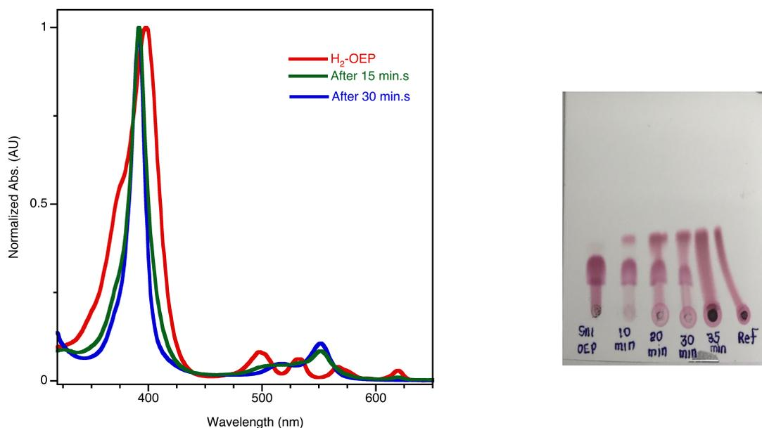
**Figure S2.** Left: UV-vis spectrum (CH<sub>2</sub>Cl<sub>2</sub>) of **[OEP]Co** in comparison to that of the corresponding free base **OEP** over the reaction time. Right: representative TLC image used to judge the progress of the metal insertion reaction (silica-ethyl acetate:hexanes:MeOH-55:40:5).
