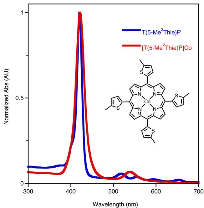
**Figure S26.** UV-vis spectrum (CH<sub>2</sub>Cl<sub>2</sub>) of [T(5-Me<sup>2</sup>Thie)P]Co in comparison to that of the corresponding free base T(5-Me<sup>2</sup>Thie)P. [T(5-Me<sup>2</sup>Thie)P]Co is literature-known.<sup>4</sup>
