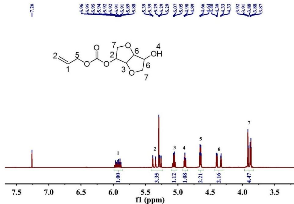
Figure S15.  $^1\text{H}$  NMR spectrum of **2b'**
