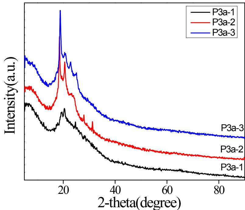
Figure S66. Comparative XRD patterns of polycarbonate with different chain lengths from click chemistry
