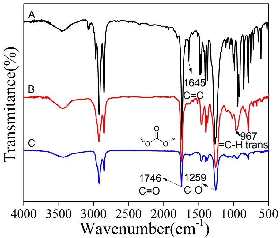
Figure S64. FT-IR spectra of **2a-3** (A), **P4a-3** (B) and **PH4a-3** (C).
