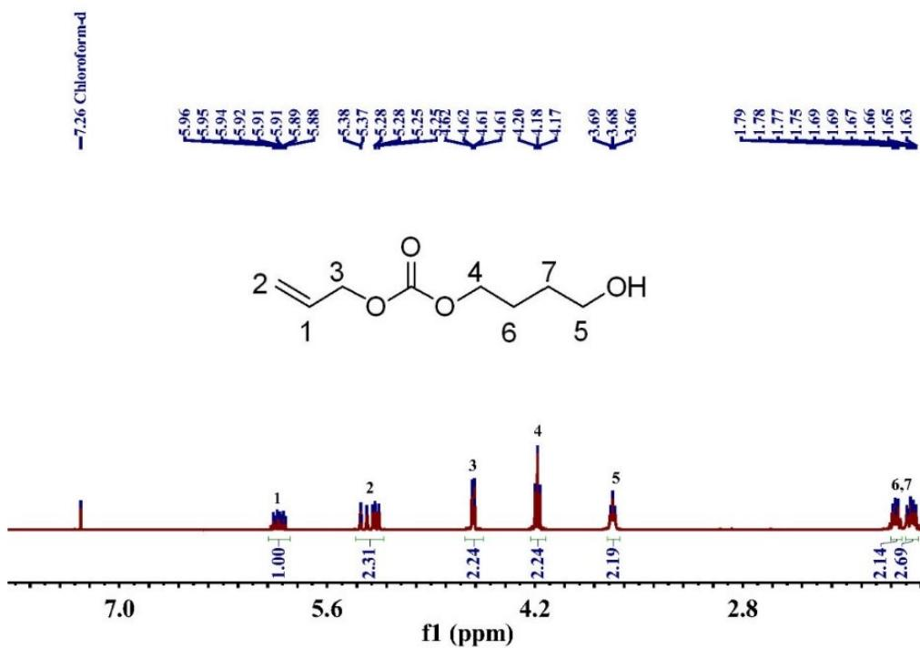
Figure S23.  $^1\text{H}$  NMR spectrum of **2d'**
