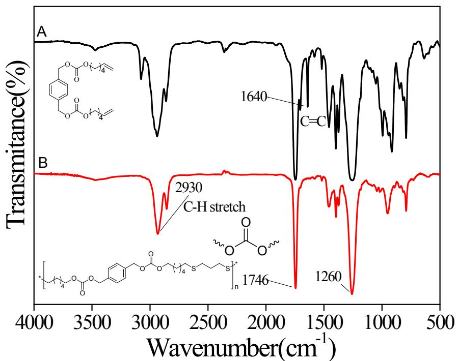
Figure S54. FT-IR spectra of **2a-2** (A) and **P3a-2** (B)
