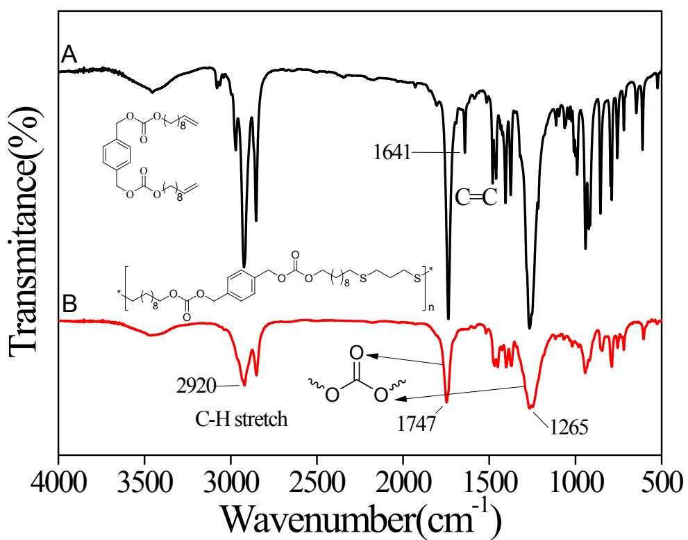
Figure S55. FT-IR spectra of **2a-3** (A) and **P3a-3** (B)
