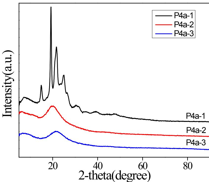
Figure S69. Comparative XRD patterns of polycarbonate with different chain lengths from ADMET polymerization
