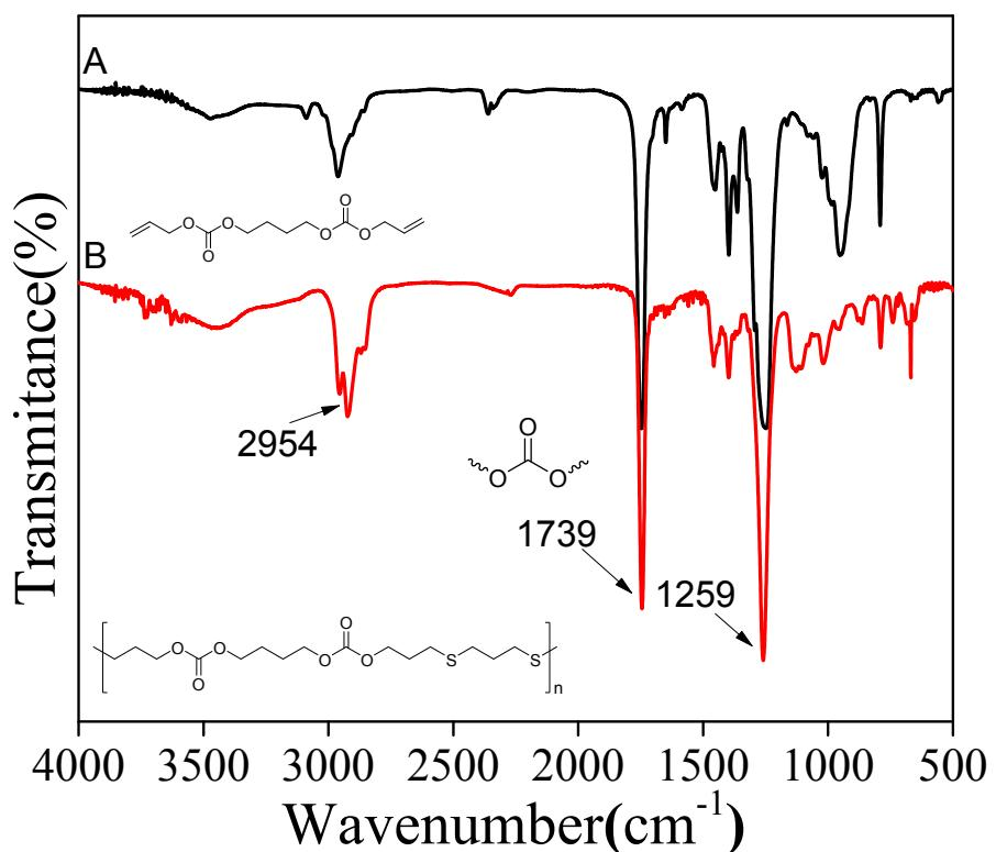
Figure S59. FT-IR spectra of **2d** (A) and **P3d** (B)
