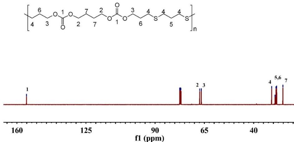
Figure S41.  $^{13}\text{C}$  NMR spectrum of P3d
