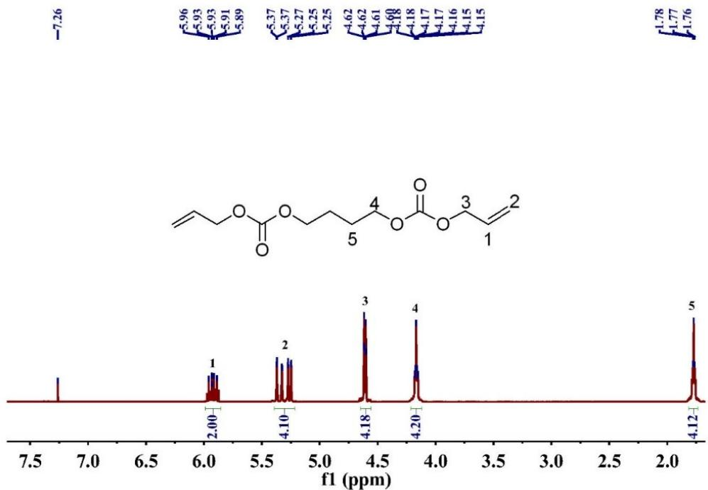
Figure S21.  $^1\text{H}$  NMR spectrum of **2d**
