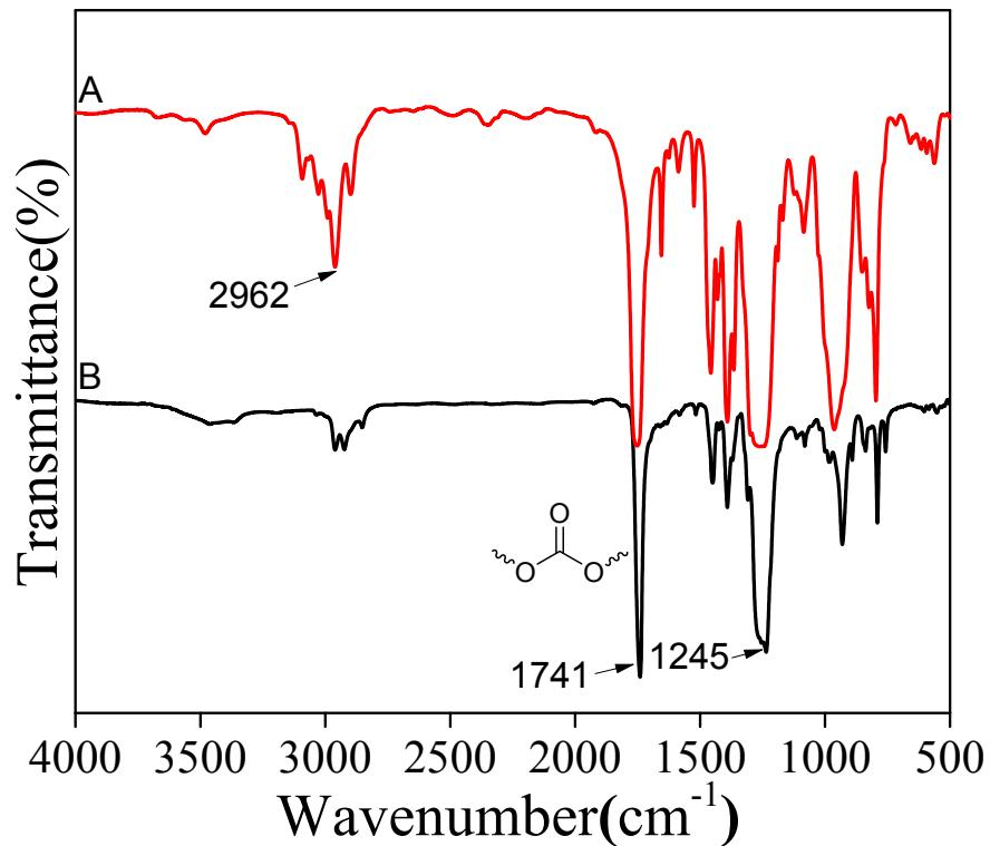
Figure S62. FT-IR spectra of **2a-1** (A) and **P4a-1** (B)
