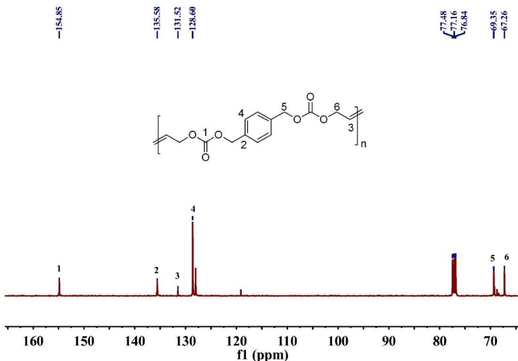
Figure S45.  $^{13}\text{C}$  NMR spectrum of P4a-1
