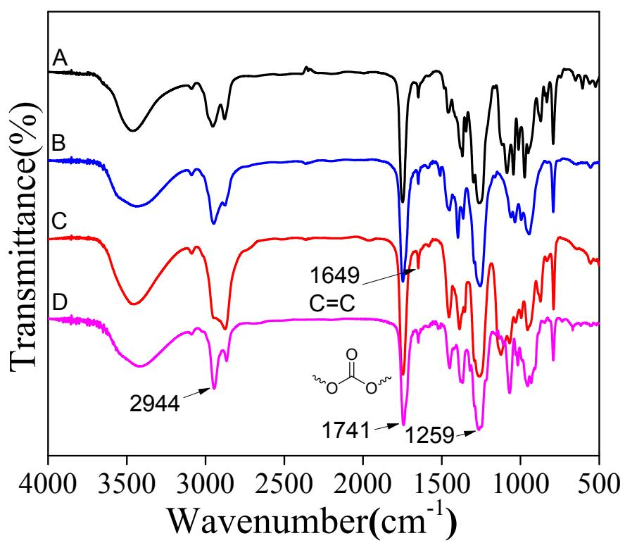
Figure S61. FT-IR spectra of **2b'** (A), **2c'** (B), **2d'** (C) and **2e'** (D)
