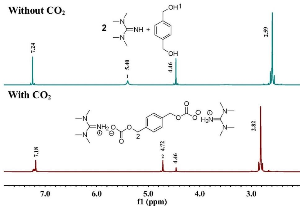
Figure S52. Comparative <sup>1</sup>H NMR spectra of TMG–BDM (2:1, molar ratio) in d<sub>6</sub>-DMSO without and with CO<sub>2</sub> addition. A new signal assigned to the carbonate carbon appeared at  $\delta = 156.2$  ppm after CO<sub>2</sub> addition, which indicated the formation of 2[TMGH]<sup>+</sup>[O<sub>2</sub>COCH<sub>2</sub>C<sub>6</sub>H<sub>4</sub>CH<sub>2</sub>OCO<sub>2</sub>]<sup>2-</sup>.
