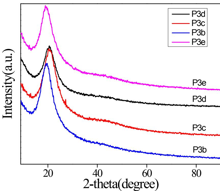
Figure S68. Comparative XRD patterns of polycarbonate from different diols from click chemistry
