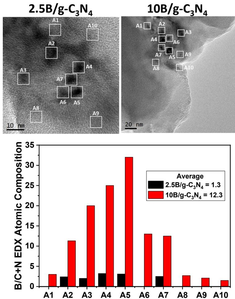
Figure S2. TEM-EDX analysis of 2.5B/g-C<sub>3</sub>N<sub>4</sub> and 10B/g-C<sub>3</sub>N<sub>4</sub> samples.
