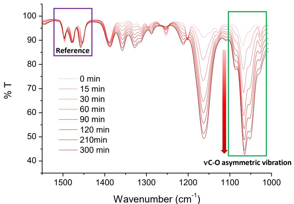
**Figure S5.** Partial FT-ATR-IR spectra used to obtain the kinetic profiles for the reaction between styrene oxide (**6**) and CO<sub>2</sub> to afford **7**. Reaction conditions: solventless, 100 °C, 5 h, CO<sub>2</sub> balloon.
