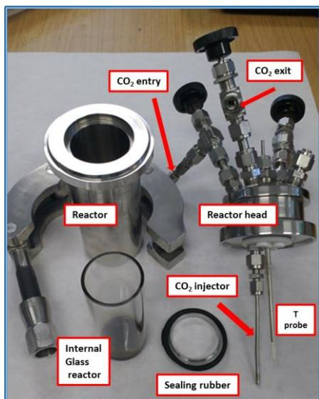
**Figure S11.** Reactor set-up used to perform the cycloaddition reaction under CO<sub>2</sub> pressure.
