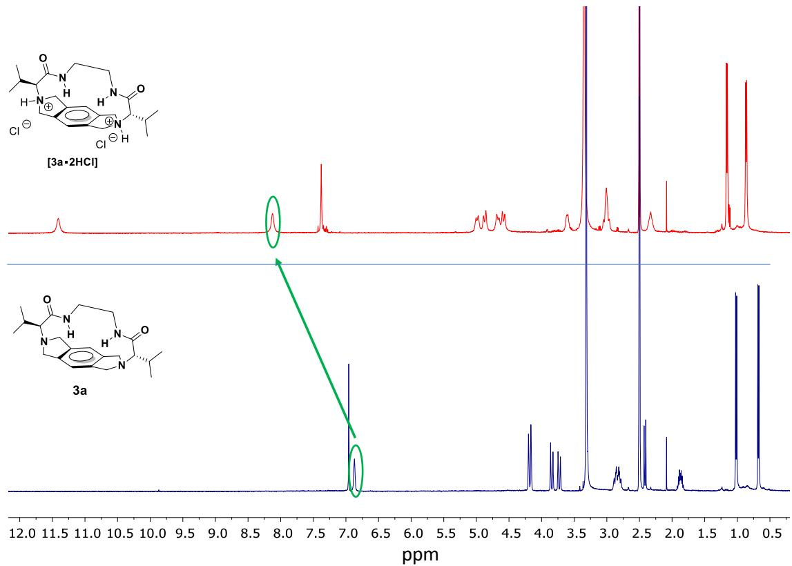
**Figure S6.** <sup>1</sup>H NMR (400 MHz, 30 °C) spectra of **3a** and **[3a·2HCl]** using DMSO-d<sub>6</sub> as the solvent (9 mM). The downfield shift observed for the NH<sub>amide</sub> has been highlighted in green.
