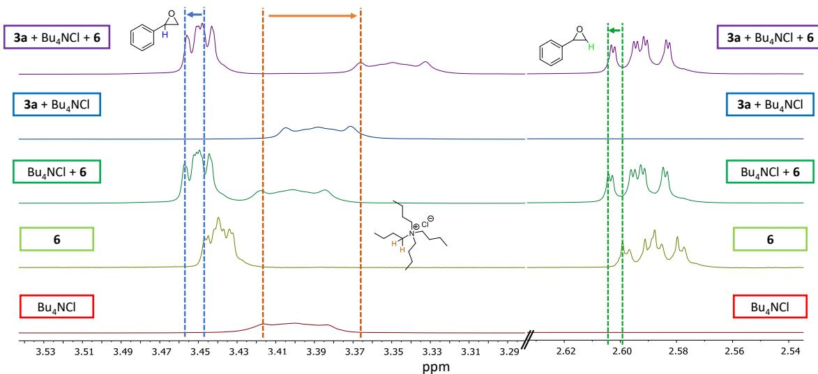
**Figure S8.** Partial  $^1\text{H}$  NMR (500 MHz) spectra for  $\text{Bu}_4\text{NCl}$ ,  $6$  and the mixtures  $[\text{Bu}_4\text{NCl} + 6]$ ,  $[\text{3a} + \text{Bu}_4\text{NCl}]$  and  $[\text{3a} + \text{Bu}_4\text{NCl} + 6]$  in  $\text{C}_6\text{D}_6$ .  $[6] = 240 \text{ mM}$ ;  $[\text{Bu}_4\text{NCl}] = 20 \text{ mM}$ ;  $[\text{3a}] = 2 \text{ mM}$  (samples in 1 mL of  $\text{C}_6\text{D}_6$ ).
