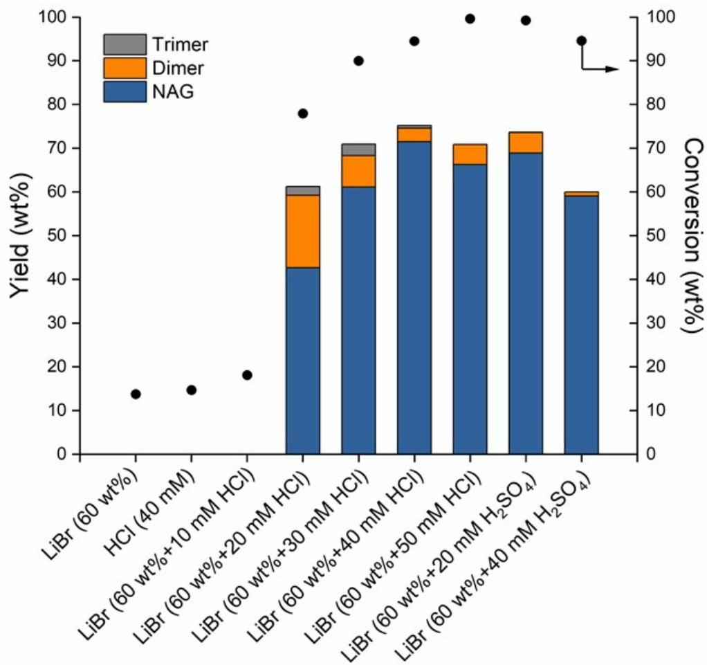
**Fig. S1** Conversion and monomers/oligomers' yields from chitin with different concentrations of HCl and H<sub>2</sub>SO<sub>4</sub>. Reaction conditions: 0.2 g chitin and 4 mL LiBr AMSH at 120 °C for 30 min.
