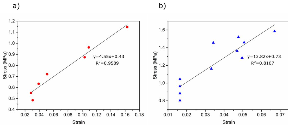
Fig. S7. Stress–strain curves determined for a) DCC\_2.5 and b) NCC\_2.5.
