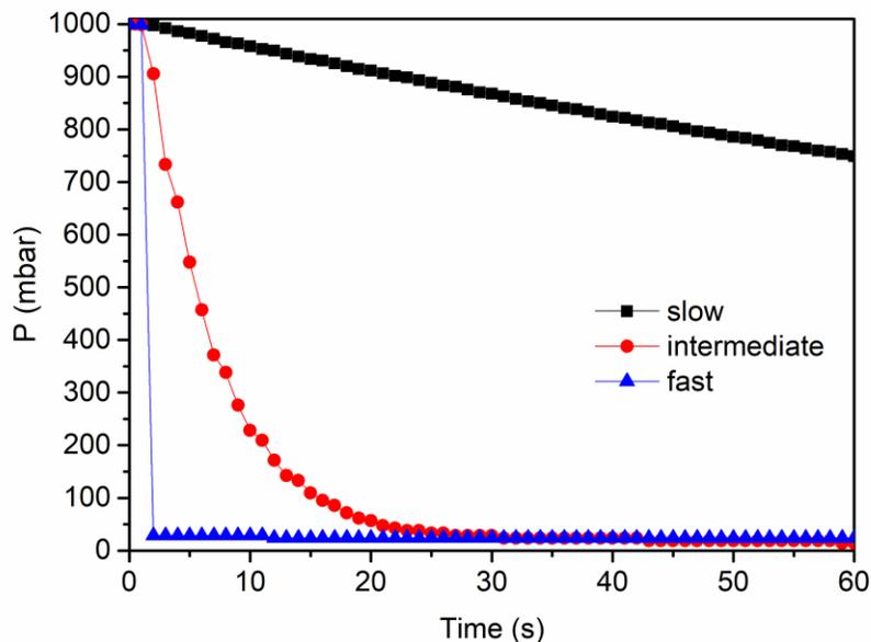
Fig. S5. Decrease in ambient pressure in the sample chamber over time at different positions of the leak valve. To perform the experiments, a pressure of 1 mbar was set in the pre-chamber, next the leak valve was opened and the time needed to reach the equilibration pressure was measured.
