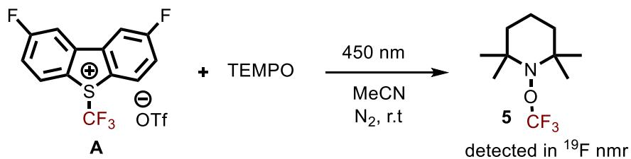
A mixture of Umemoto reagent II (**A**) (19.7 mg, 0.045 mmol) and TEMPO (7 mg, 0.045 mmol) in CH<sub>3</sub>CN was irradiated in PR m2 (blue LED, 450 nm) for 4 hours. The reaction mixture was concentrated and dissolved in CDCl<sub>3</sub> to record <sup>19</sup>F nmr. CF<sub>3</sub>-TEMPO adduct was detected in an yield of 40% (using trifluorotoluene as internal standard) in <sup>19</sup>F nmr.
