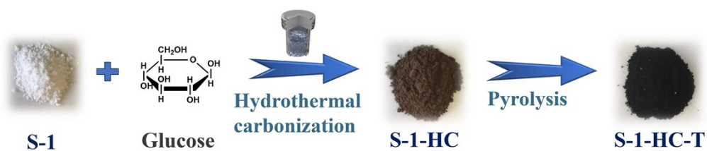
Scheme S1. Graphical illustration of the synthesis route for the S-1-HC-T nanocomposites.
