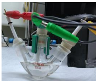
Figure S23. The digital graph of the setup of the electrochemical cell for Figure 1.
