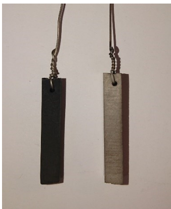
Fig. S4: Digital photograph of a carbon rod cathode, unmodified (left) and NiMo-coated via electroplating (right).
