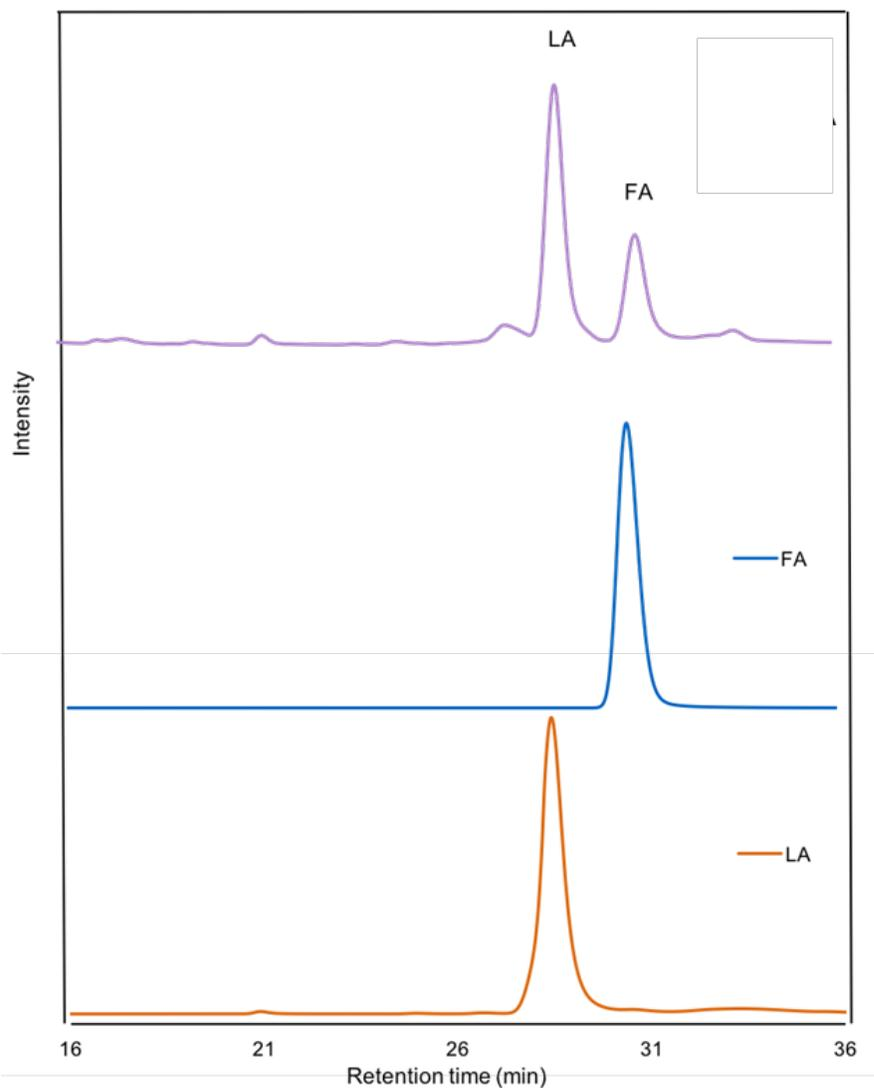
**Figure S6.** Typical HPLC chromatogram at 218 nm wavelength against authentic formic acid (FA), lactic acid (LA).
