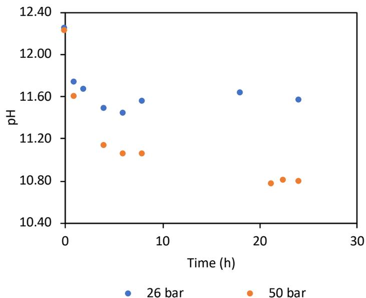
**Figure S5.** Comparison of changes in pH observed in the reaction of glycerol using catalyst **7**, 6.85 M aqueous glycerol, 2.70 M  $K_2CO_3$ , 0.001 mol% **7**, 150 °C,  $N_2$  pressure of 26 bar and 50 bar.
