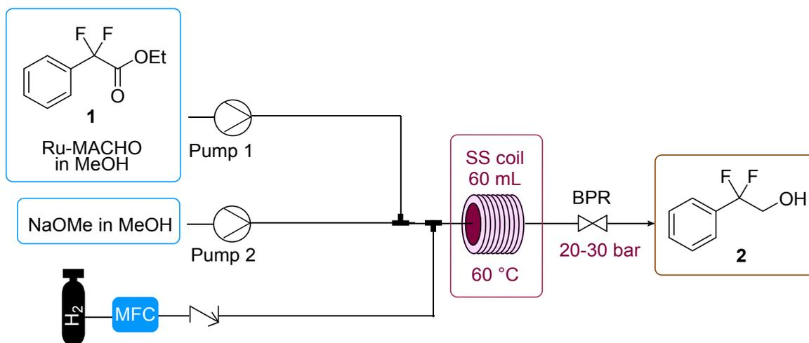
**Scheme S1.** Continuous flow scheme for the Ru-MACHO hydrogenation optimization experiments.
