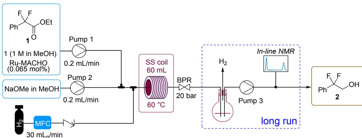
**Scheme S2.** Continuous flow scheme for the Ru-MACHO hydrogenation long run.
