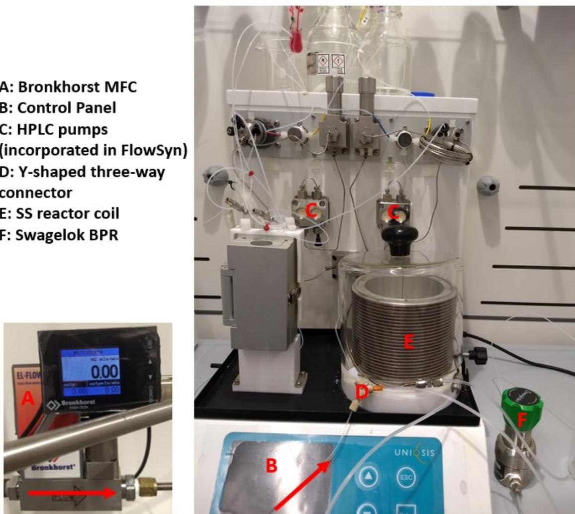
**Figure S1.** Labeled continuous flow setup for the Ru-MACHO hydrogenation optimization experiments.
