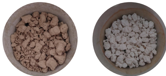
Figure 2: Residues of lignins after oxidation. Left: residues from lignin/attapulgite mixture. Right: residues from lignin with calcium hydroxide.
