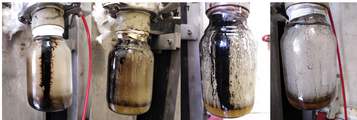
Figure 8: Visualization of pyrolysis liquids from fast pyrolysis of lignins. From left to right: pure lignin, lignin/attapulgite, lignin-calcium hydroxide and lignin/sodium formate.
