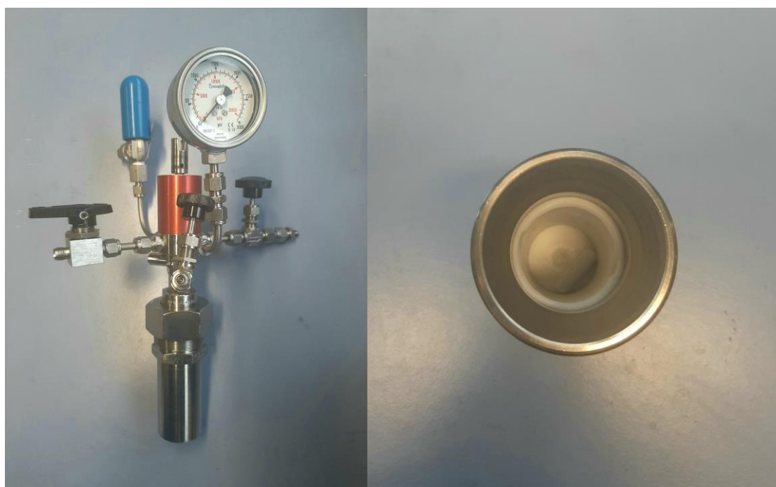
Figure 6 Representative picture of a Premex autoclave used in high pressure reaction.
