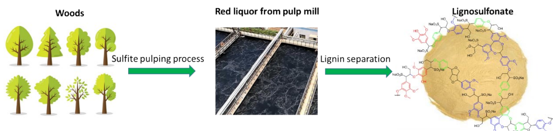
Figure. S1 Lignosulfonate from the spent liquor (red liquor) of the sulfite pulping process and its structure.
