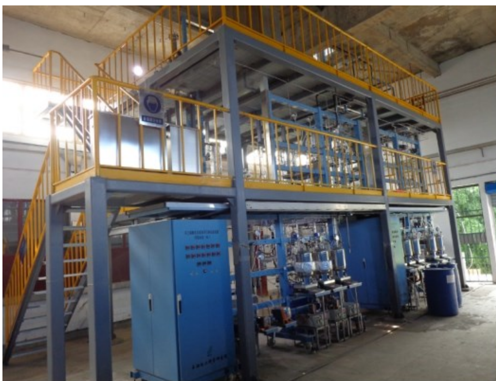
Fig. S7 The flow chart (top) and photograph (bottom) of a pilot-scale reactor with a reactive-distillation reactor in conjugation with a fixed-bed reactor for continuous cyclohexene esterification and ester hydrogenation.
