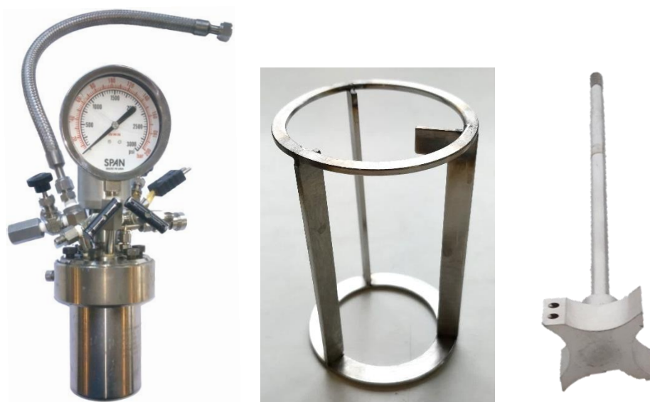
Figure S2: 350 mL stirred tank reactor (left), baffles (middle) and gas-impeller stirrer (right)
