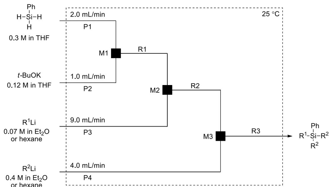
A microfluidic system consisting of three T-shaped micromixers (M1, M2 and M3), three tube reactors (R1, R2 and R3) and four tube pre-temperature-retaining units (for P1, P2, P3 and P4,  $\phi = 1$  mm and  $L = 100$  cm) were used. The microfluidic system was immersed in a temperature control bath. A solution of phenylsilane (0.3 M in
