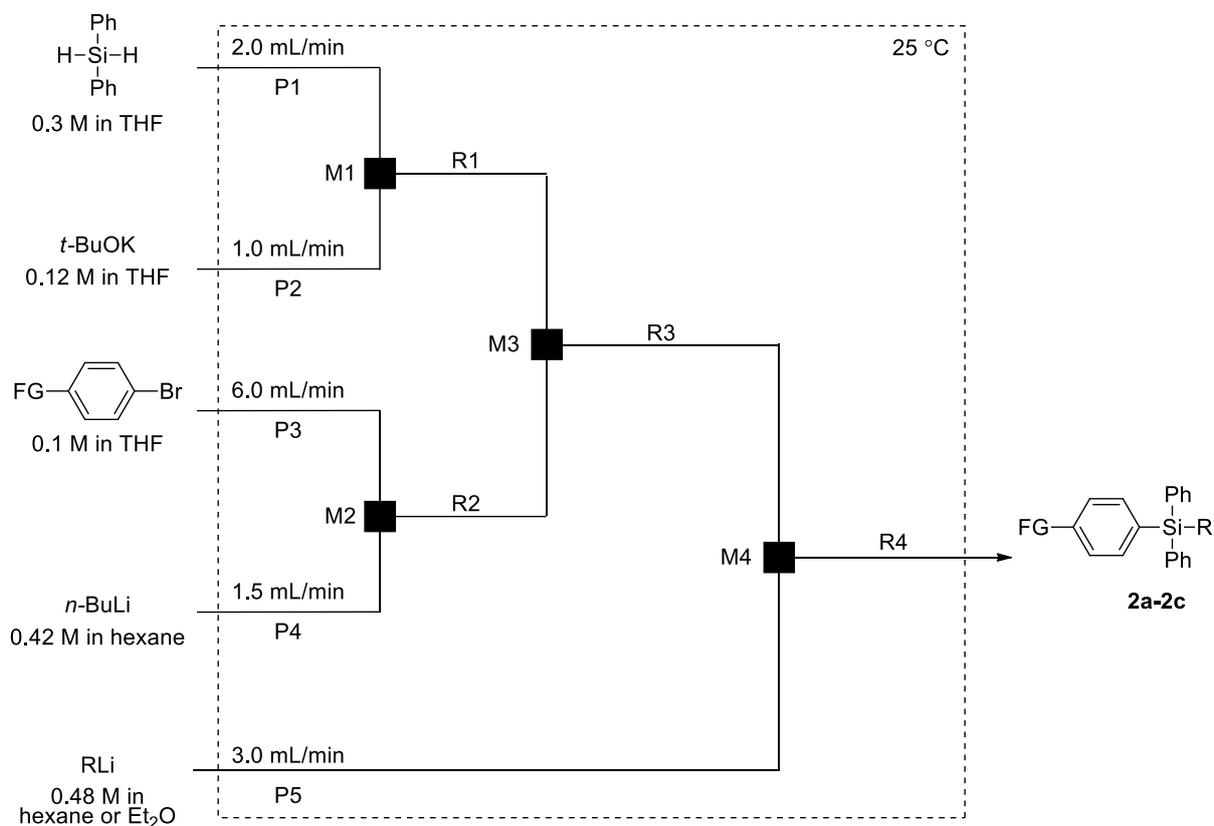
A microfluidic system consisting of four T-shaped micromixers (M1, M2, M3 and M4), four tube reactors (R1, R2, R3 and R4) and five tube pre-temperature-retaining units (for P1, P2, P3, P4 and P5,  $\phi = 1$  mm and  $L = 100$  cm) were used. The microfluidic system was immersed in a temperature control bath. A solution of diphenylsilane
