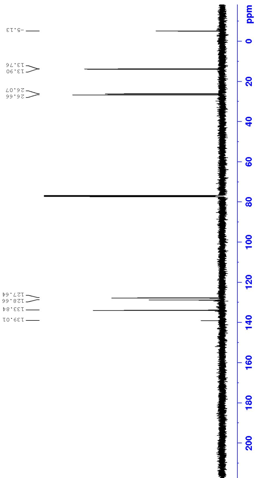
$^{29}\text{Si}$  NMR spectra of **dibutyl(methyl)(phenyl)silane (3d)**
