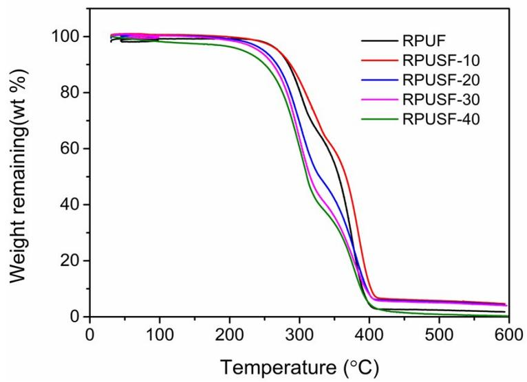
**Fig. S7** TGA curves of the RPUF and RPUSFs.
