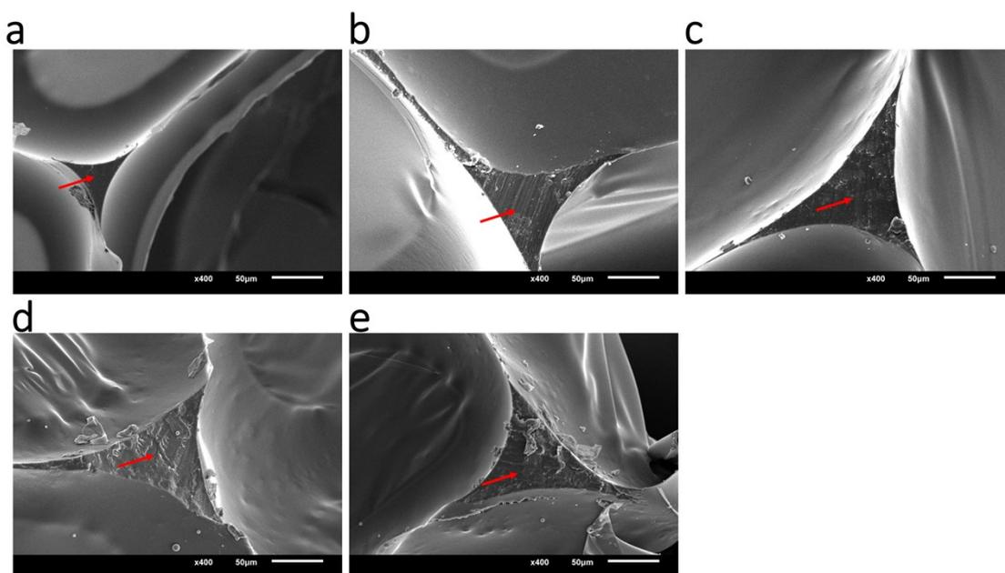
**Fig. S2** SEM images with ×400 magnification of PUF (a), PUSF-10 (b), PUSF-20 (c), PUSF-30 (d), and PUSF-40 (e) showing the size of strut joint (as designated with red arrow).
