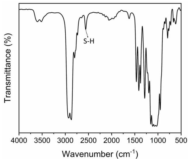
**Fig. S1** FT-IR spectrum of polysulfide oligomer (PSO).
