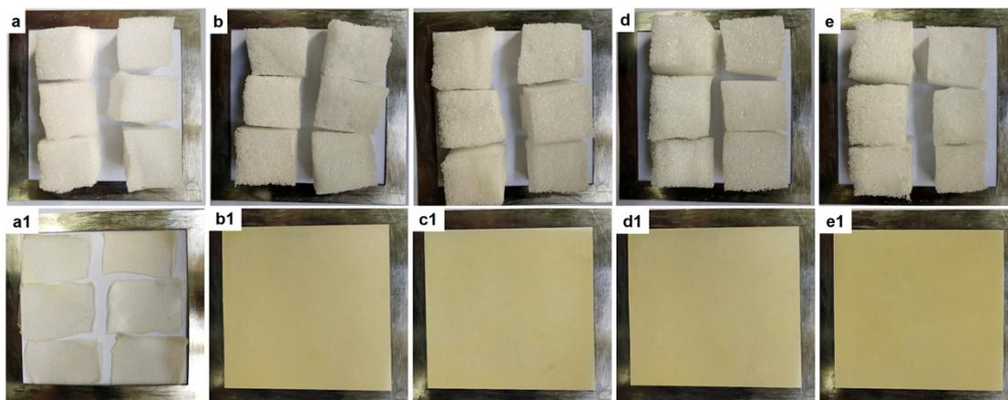
**Fig. S3** The photographs of original PU foams: PUF (a), PUSF-10 (b), PUSF-20 (c), PUSF-30 (d), and PUSF-40 (e) and of the recycled PU films: RPUF (a1), RPUSF-10 (b1), RPUSF-20 (c1), RPUSF-30 (d1), and RPUSF-40 (e1).
