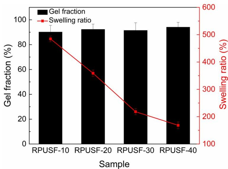
**Fig. S4** Gel fraction and swelling ratio of recycled PU films from malleable PU foams with different compositions.
