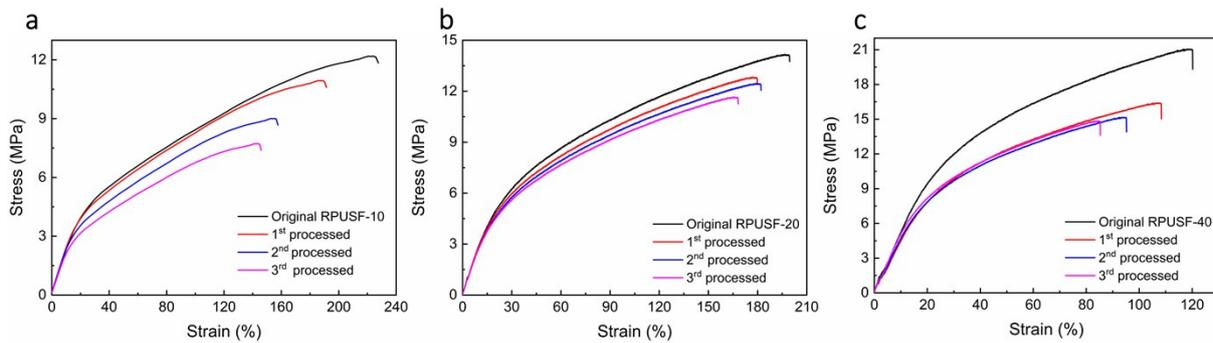
**Fig. S5** Stress-strain curves of original and reprocessed RPUSF-10 (a), RPUSF-20 (b), and RPUSF-40 (c).
