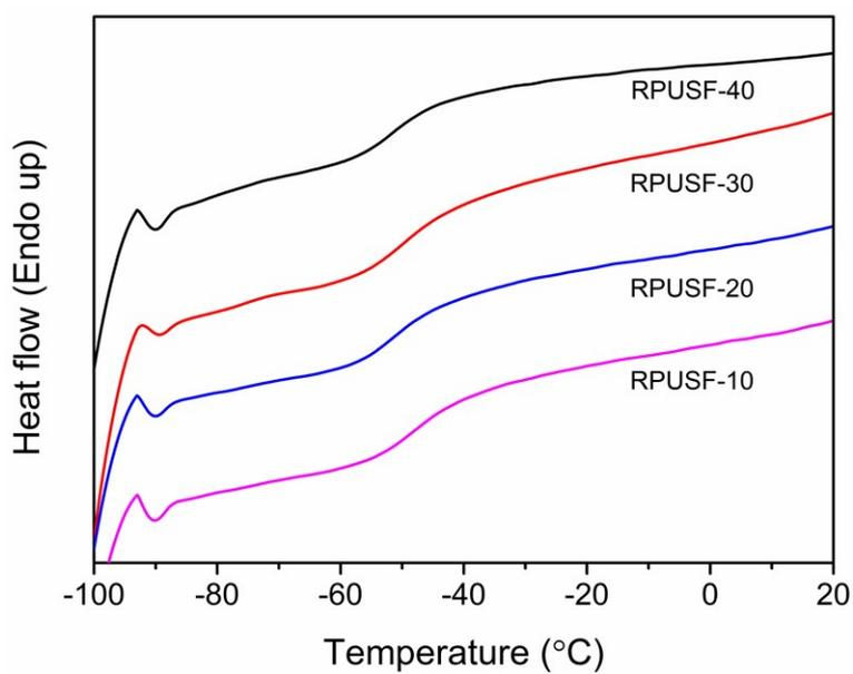
**Fig. S6** DSC heating scans of RPUSFs.
