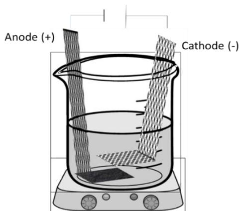
**Figure S2:** Schematic representation of the cell used for bulk electrochemical dissolution of metal oxides in DES media. A slurry of the metal oxide is pasted onto the anode.
