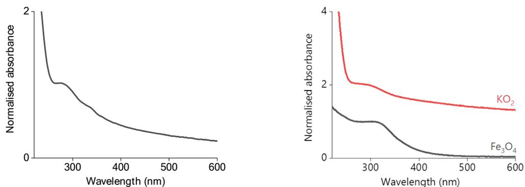
**Figure S5:** UV-Vis spectra of solution of KO<sub>2</sub> after chemical dissolution in EG:ChCl (left), and compared to the solution obtained from anodic dissolution of Fe<sub>3</sub>O<sub>4</sub> (right).
