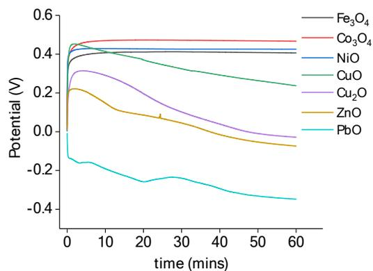
**Figure S1:** Open circuit potential of metal oxides paint casted in EG:ChCl, with a 0.32 cm<sup>2</sup> Pt flag WE, a Pt flag CE and an Ag/AgCl (0.1 M in EG:ChCl) reference electrode.
