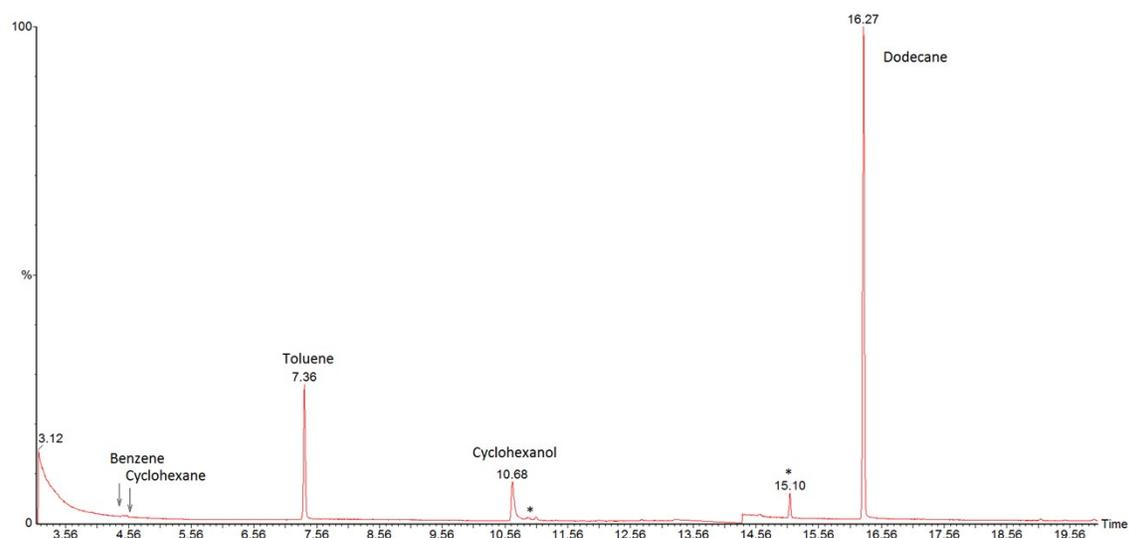
Figure S4. Example of chromatogram. In this case resulting from the catalysis of benzyl phenyl ether. Marked with a \* the signals derived from solvent.
