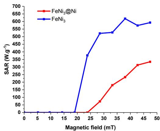
Figure S2. Specific Absorption Rate measured as a function of the applied field ( $\mu_0 H_{rms}$ ) and for a fixed frequency of 93 kHz for FeNi<sub>3</sub> (in blue) and FeNi<sub>3</sub>@Ni NPs (in red).<sup>1</sup>
