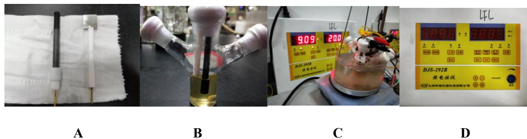
Figure S1. The experimental setup for electrolysis. (A: The electrodes used in the reaction.
