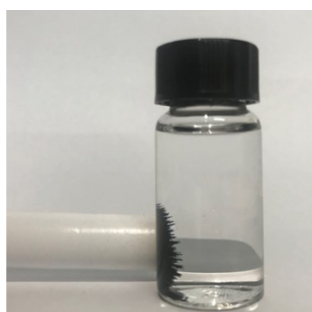
Fig. S1 The magnetic property of \text{Fe}_{10}\text{Pd}_1/\text{NC500} .
