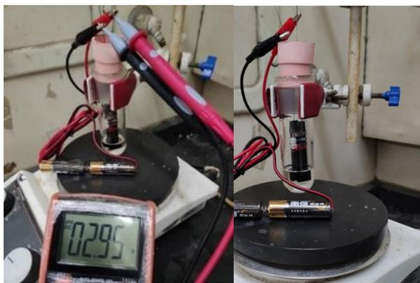
An oven-dried 10 mL undivided bottle was charged with quinoxalin-2(1H)-one (80.0 mg, 0.5 mmol, 1.0 equiv.), cyclohexylboronic acid (192.0 mg, 1.5 mmol, 3.0 equiv.), trifluoroacetic acid (150  $\mu\text{L}$ , 2.0 mmol, 4.0 equiv.),  $n\text{Bu}_4\text{NPF}_6$  (387.4 mg, 1.0 mmol, 2.0 equiv.) and DMF (5 mL). Two
