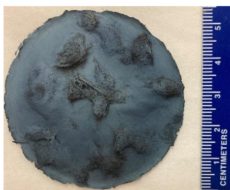
Figure S3. Film prepared using 5 wt% carbon fiber (FSE-5%). At this concentration of carbon fibers aggregation prevents further electrode fabrication.
