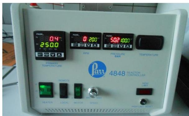
**Figure S3.** A Parr® 4848 control unit. The left screen indicates the desired (green) and actual (red) temperature (in °C) inside the reactor. The middle screen indicates the desired (green) and actual (red) stirring rate (in rpm) of the mechanical overhead stirrer, which is not used in this project. The right screen indicates the actual (red) and maximal allowed (green) pressure (in bar) before the system stops working.
