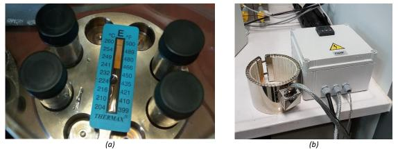
*Figure S4.* (a) A used temperature sticker, showing that the reaction media reached a temperature between 232 and 241 °C. (b) The heating system that was used for heating the Parr® 4625 reactor (IHP® Ceramic Ring Heating Mantle) (Figure S1(d)).
