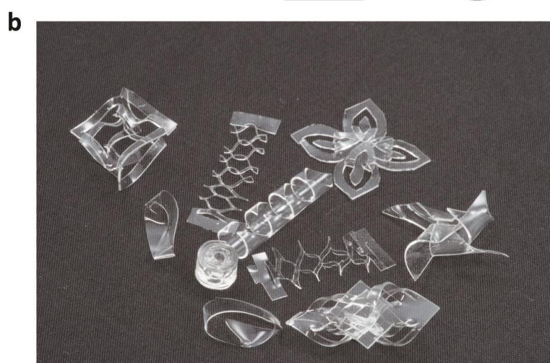
Fig. S8 Schematic of preparation of 3D structures with complex shapes (a). PDMS substrates were cut, bent, and overlapped before irradiation. Some overlapped parts were tied with polyethylene terephthalate (PET) films or paper with adhesive tapes. 3D structures produced by the proposed method (b). PDMS C films were integrated into structures with complex shapes by the hardening and bonding effects induced by a 2 MeV EB.
