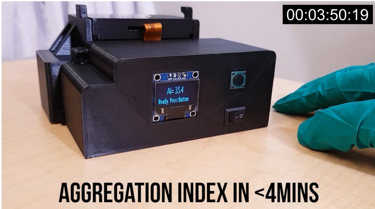
**Movie S1.** Demonstration of the CVM-based aggregometer with three simple steps; 1) turn on device, 2) load sample into chip and 3) run test. The test can be done within 4 min.
