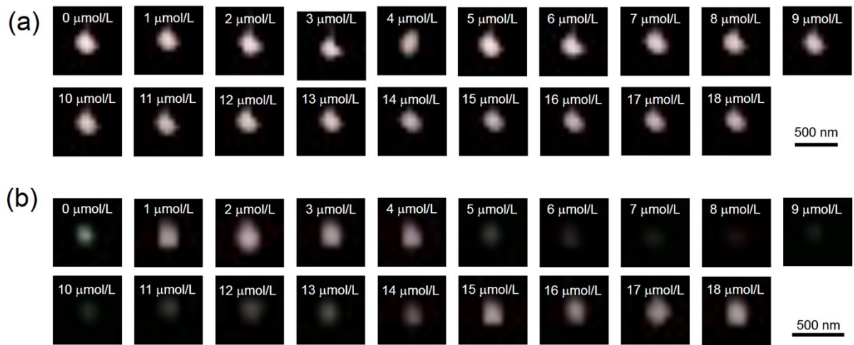
1 2 Figure S1. The output light intensity of the (a) P-MZIs and (b) unbalanced PMZI along with 3 \text{Na}_2\text{SO}_4 concentration.
