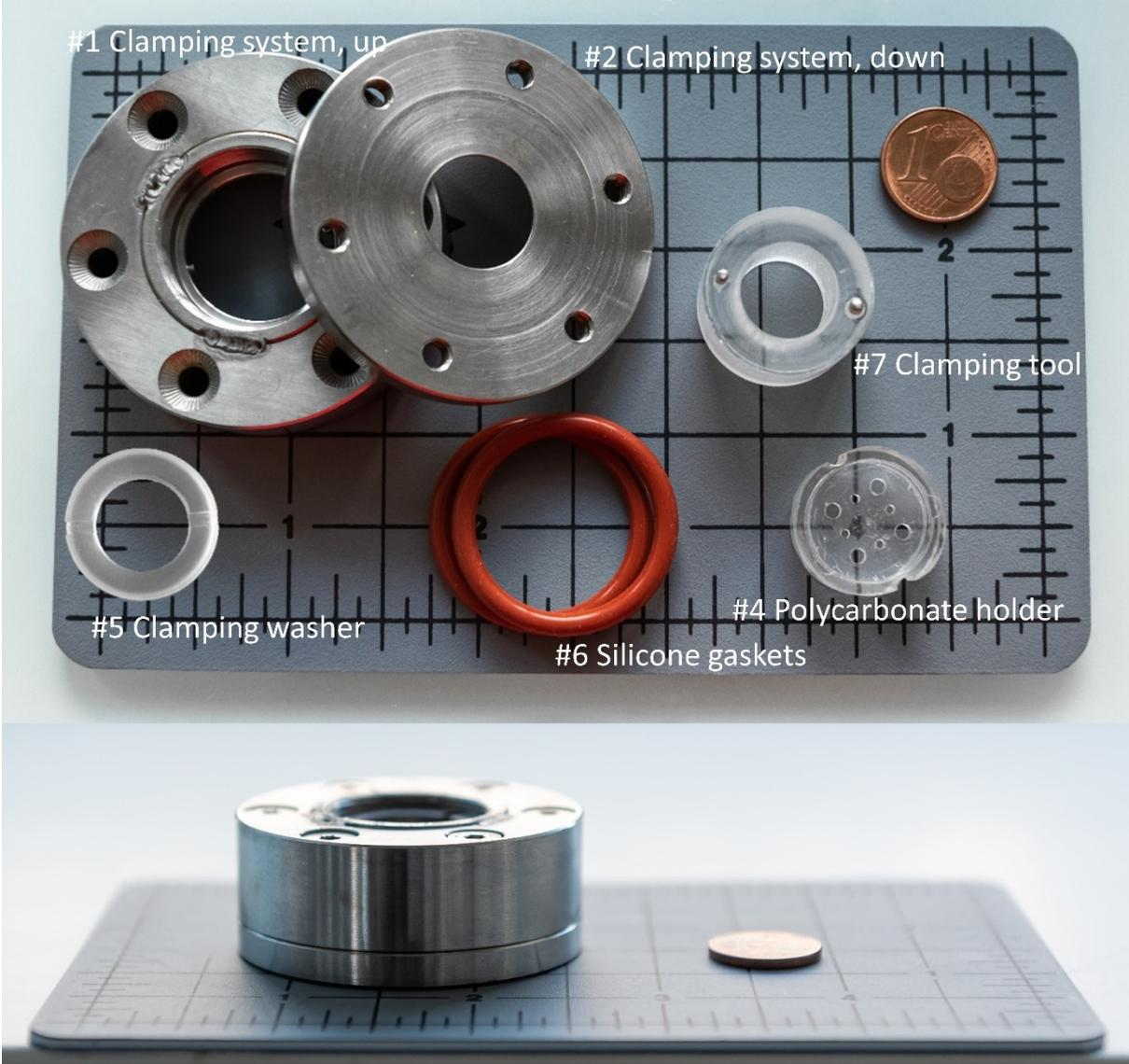
**Figure SI 2. Details on the Polycarbonate holder (Element #4 in Fig. SI 1)**
