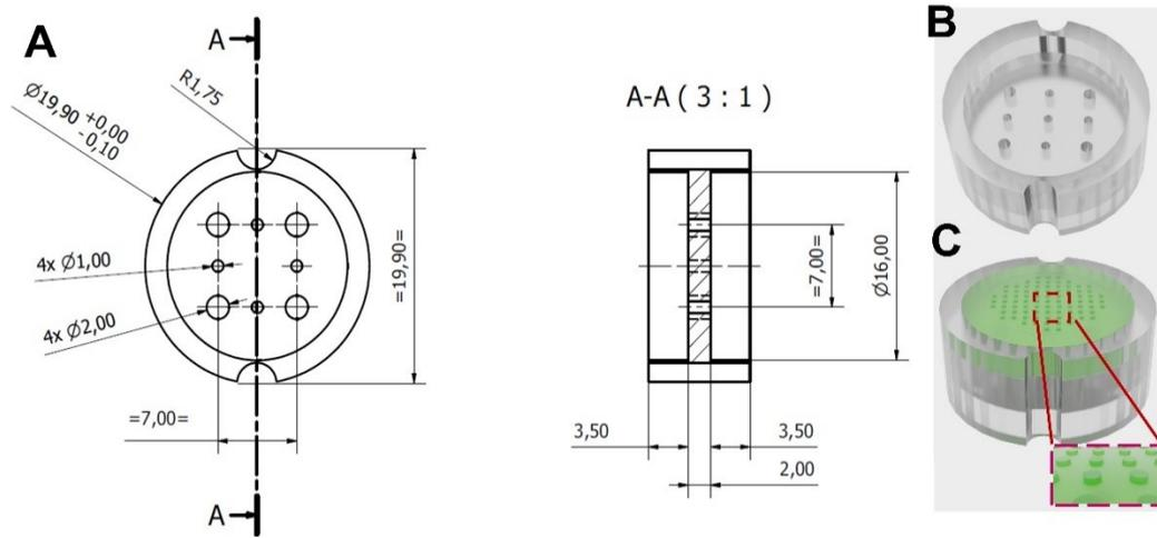
**Figure SI 3. Technical drawing (upper and side views) of the lower part of the soft confiner (Element #2 in fig. SI 1). An opening is left for microscopic viewing.**
