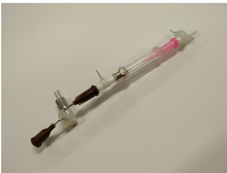
Fig. S1 Fast assembly of a DDI device with completely off-the-shelf components.
