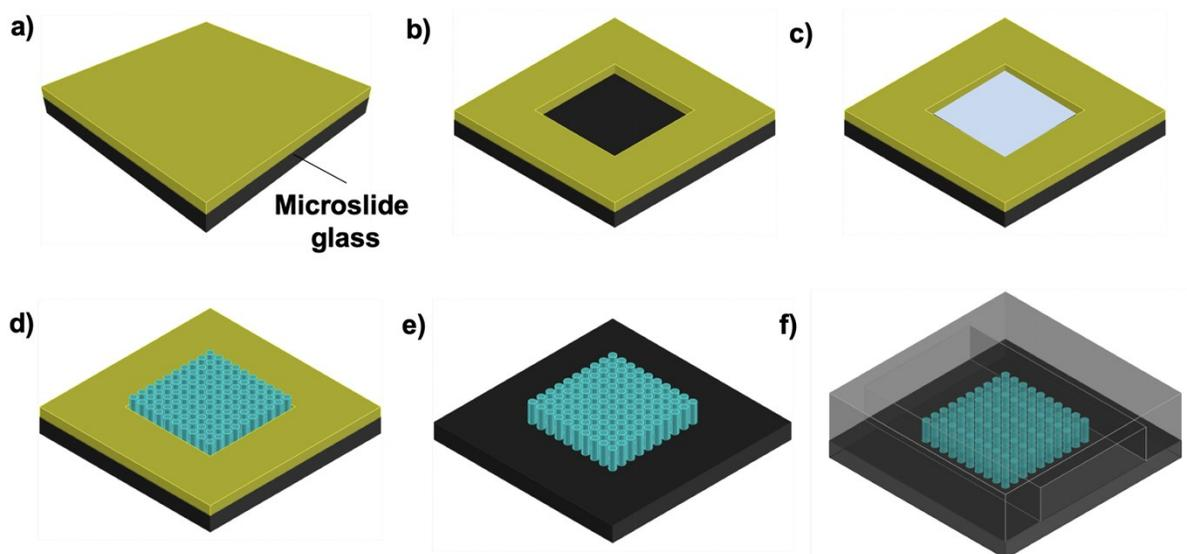
**Fig. S5** Fabrication of a microfluidic platform containing ZnO nanowires. (a) Photoresist coating. (b) Patterning (c) ZnO layer sputtering. (d) Hydrothermal growth of nanowires. (e) Photoresist removal. (f) PDMS covering.
