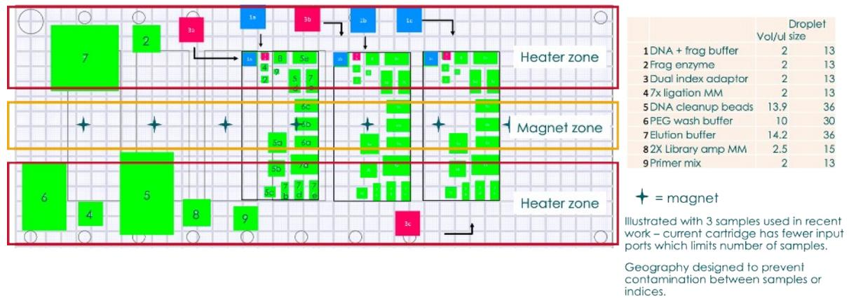
Fig. S5.6 Layout of droplets for aQdrop DNA library preparation (3 out of 6 reaction zones operating)
