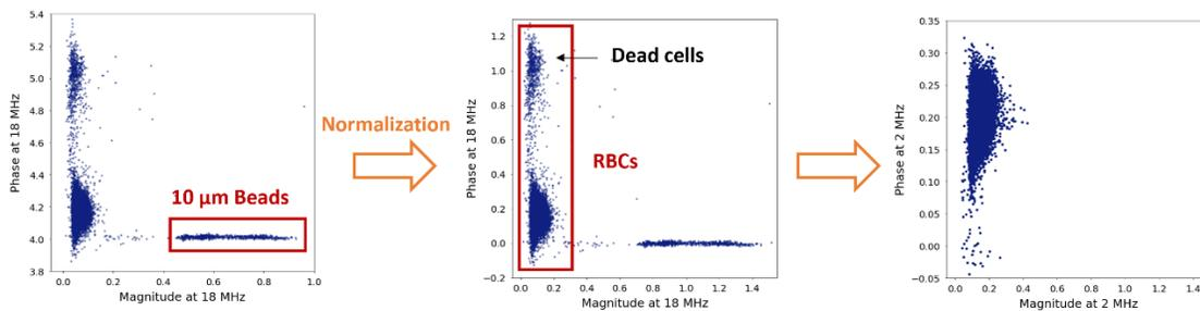
Scatter plot of impedance Magnitude versus impedance Phase at reference frequency 18 MHz is used to normalize the data against the 10  $\mu\text{m}$  polystyrene beads. After normalizing the data, a gate is then generated to include the cells. This gate is used for all the measurements at prob frequencies.
