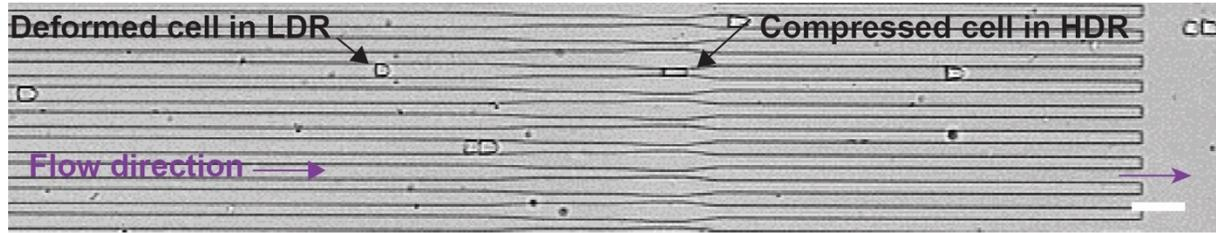
**Fig. S1** Bright field image of a microfluidic device,  $40\mu\text{m}-6\mu\text{m}$  ( $L_c-W_c$ ), showing HeLa K cells flowing through 9 microfluidic channels under an applied pressure of 5 bar. The scale bar is  $50\mu\text{m}$ .
