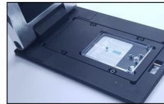
Fig S2. Schematic of customized jig for the injection molded microfluidic device (Left), Photograph of the jig connected with tubing and fitted the device (Right).
