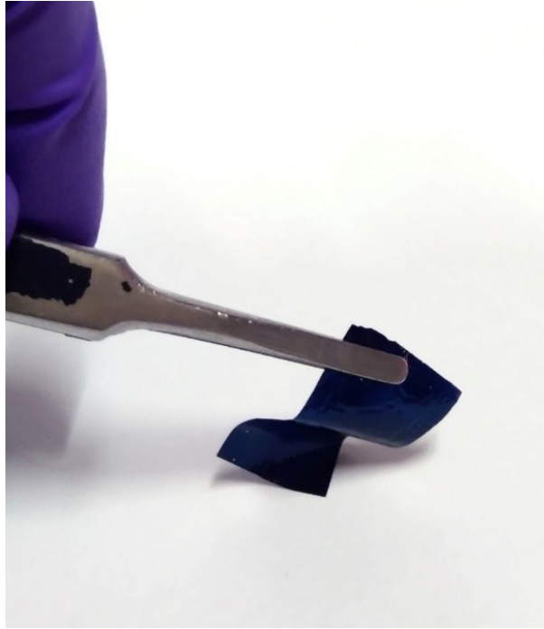
Fig.S1. optical image of the prepared flexible crosslinked PEDOT:PSS-Ti 3 C 2 T x MXene nanocomposite film.
